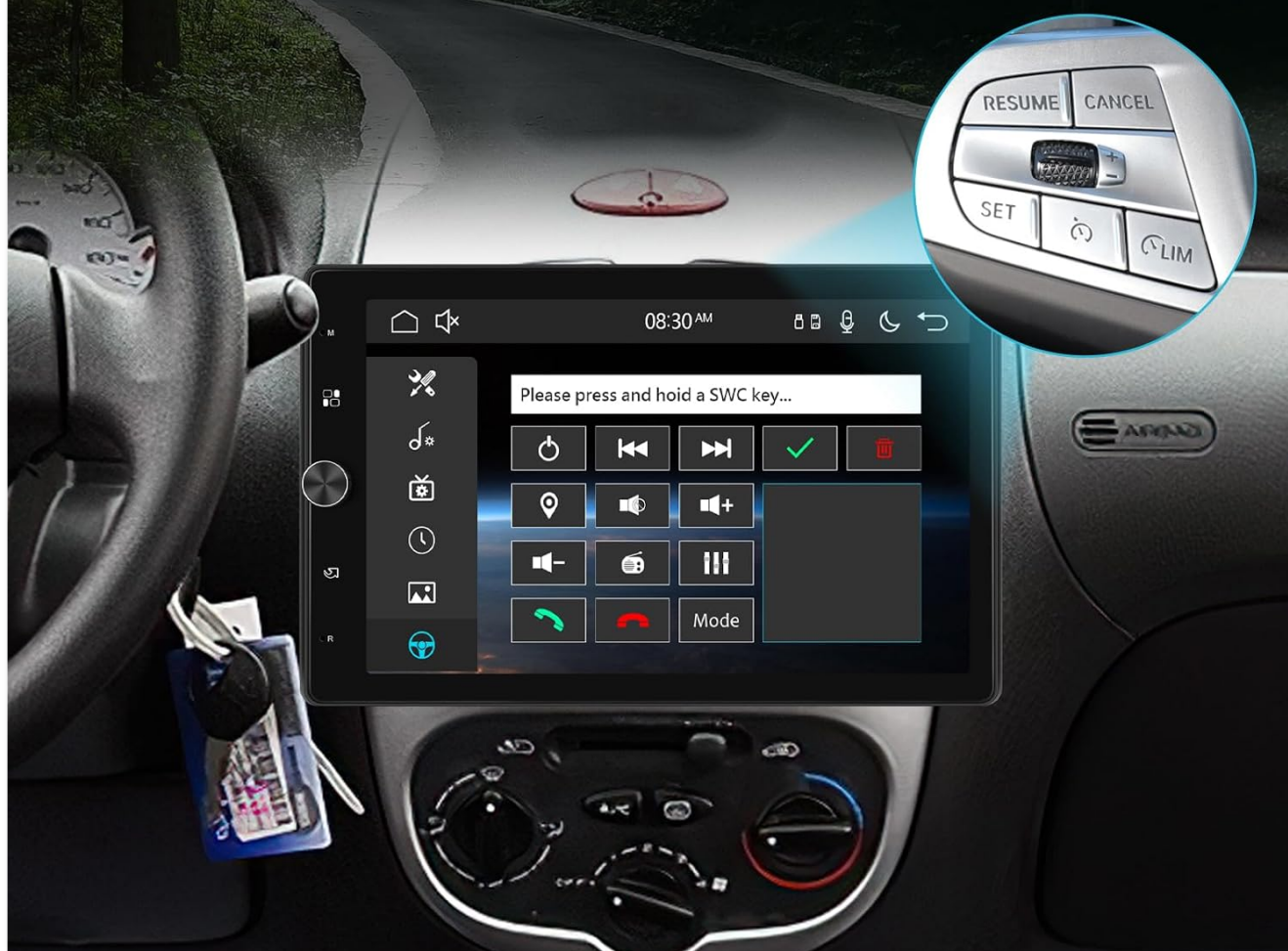
Figure 5.6: Steering Wheel Control setup. The image shows the car stereo's interface for programming steering wheel controls, allowing users to assign functions to their vehicle's existing buttons.
