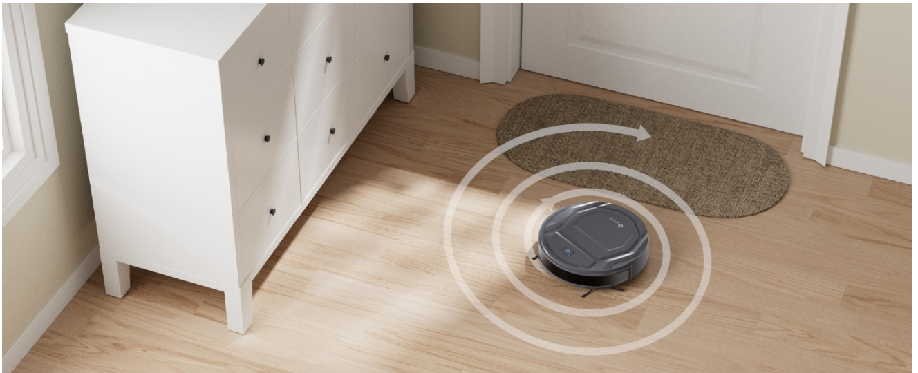
Image: A robot vacuum performing spot cleaning, moving in a spiral pattern to thoroughly clean a concentrated area.
