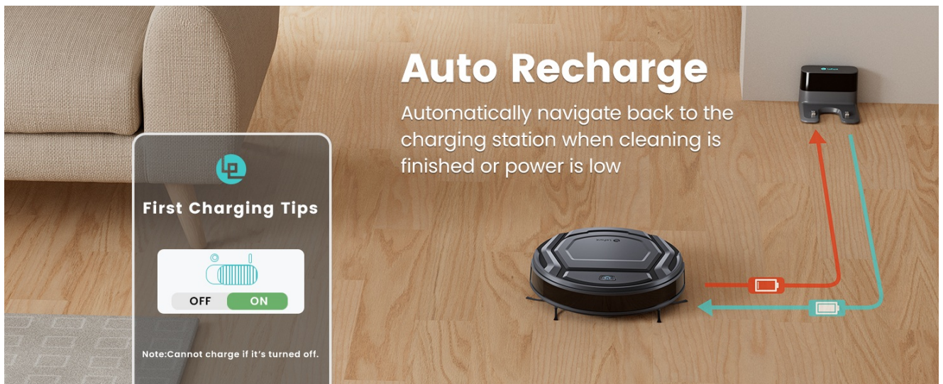
Image: A robot vacuum automatically navigating back to its charging station, demonstrating the auto-recharge feature.
