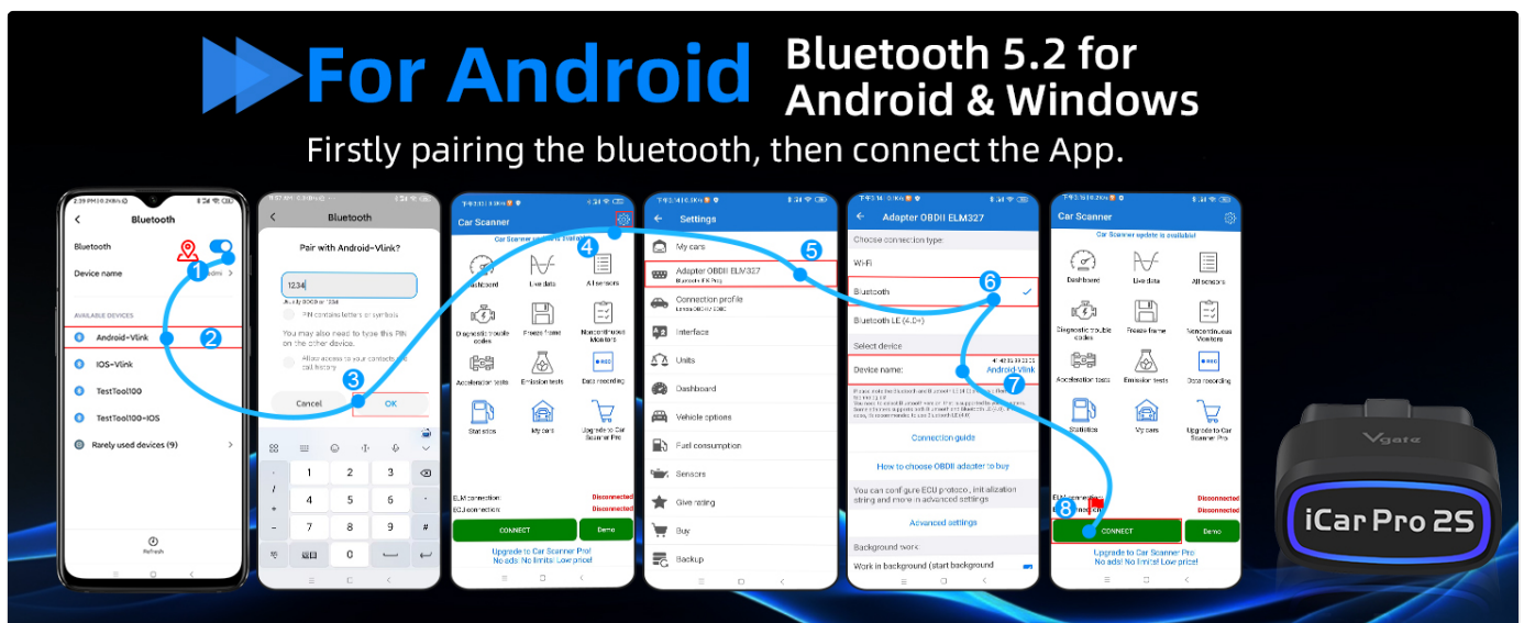
Image: Step-by-step guide for pairing and connecting the vLinker iCar Pro 2S to an Android device via Bluetooth and an OBD2 app.
