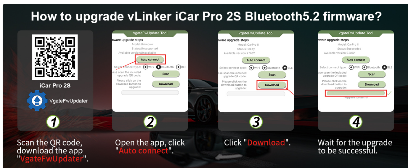
Image: Visual guide for updating the firmware of the vLinker iCar Pro 2S using the VgateFwUpdater app.
