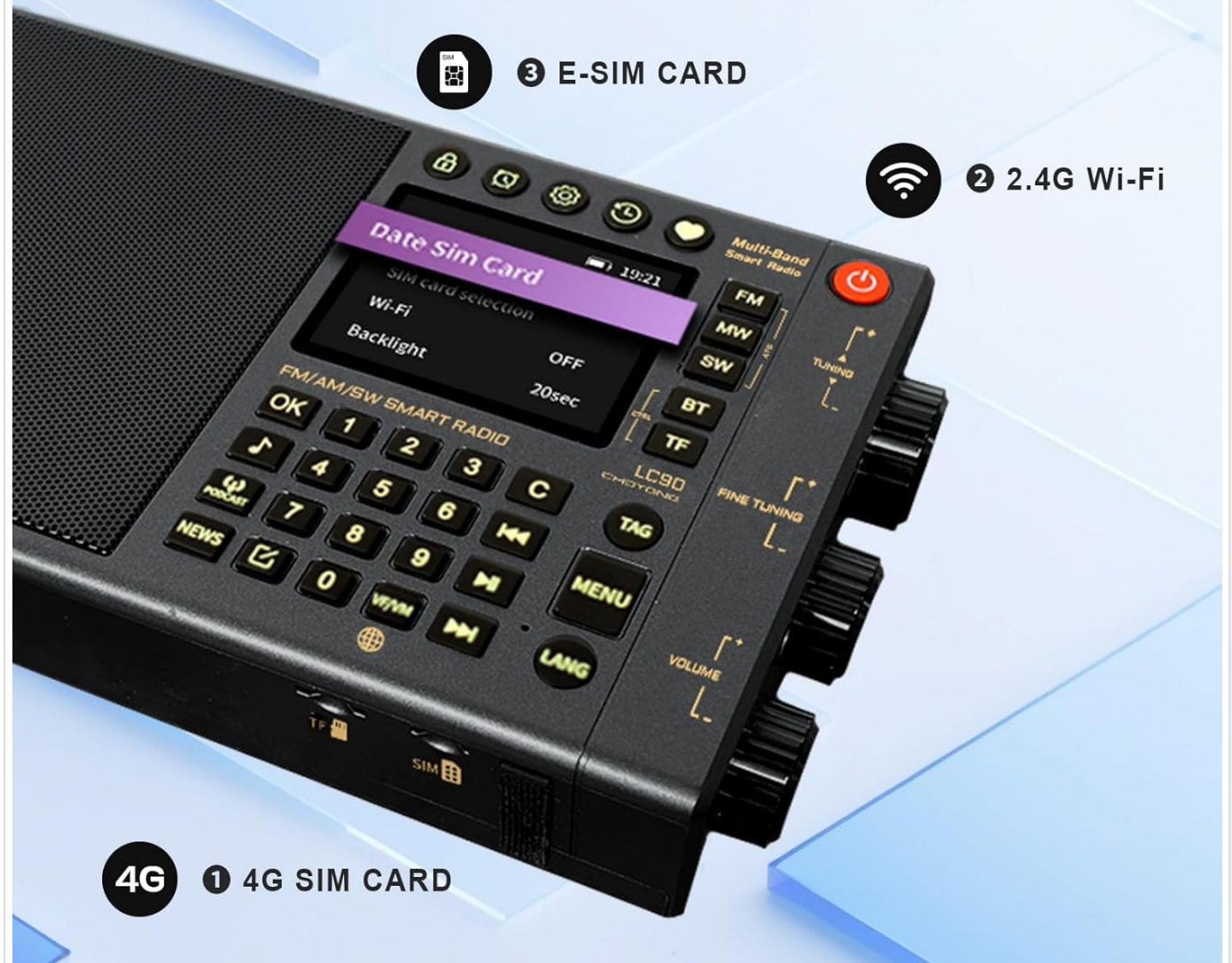
Image: Illustration of the CHOYONG LC90's networking options, including 4G SIM card, 2.4G Wi-Fi, and E-SIM card.
