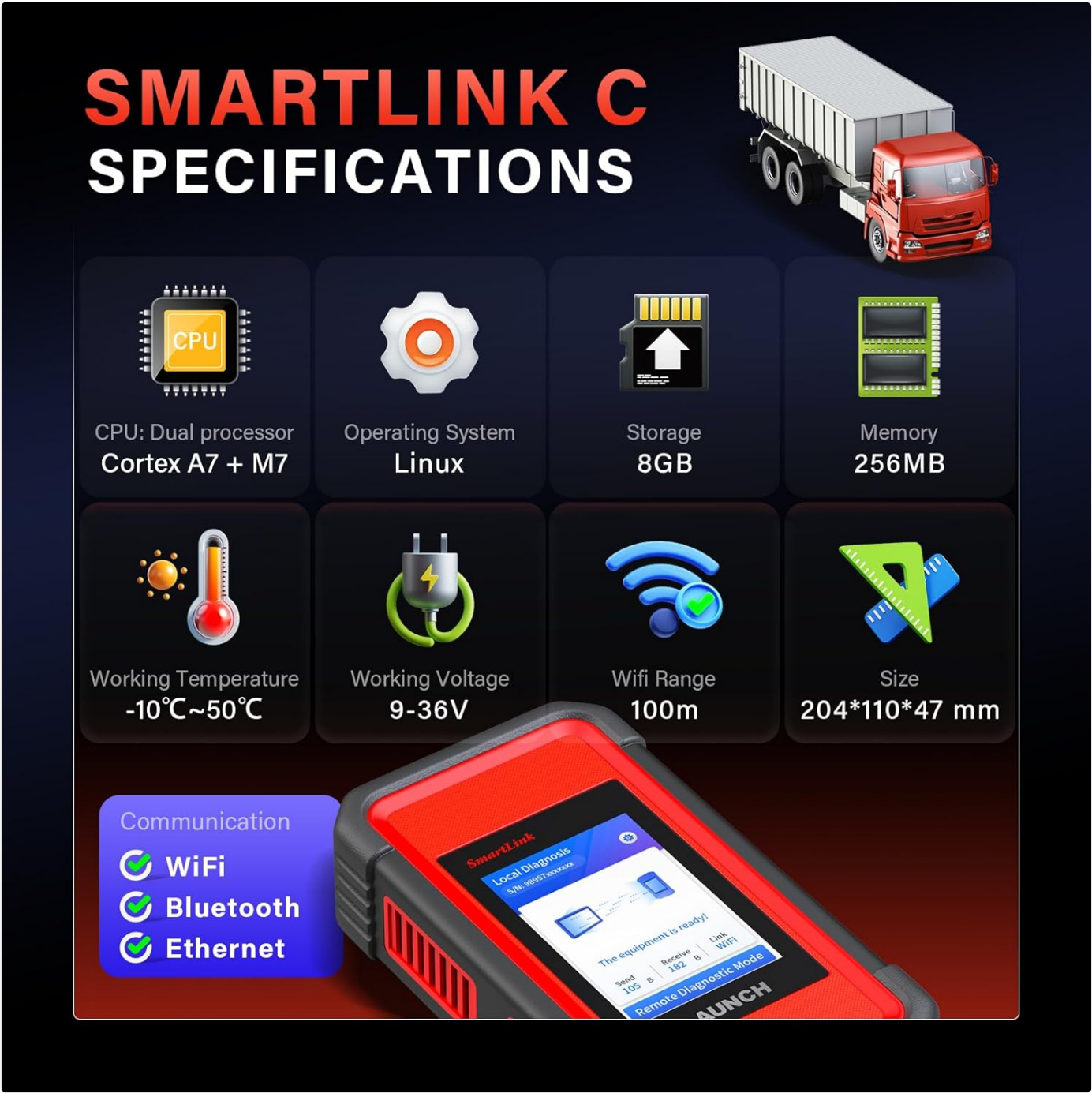
Figure 6.1: Detailed visual breakdown of the SmartLink C 2.0 specifications, including CPU, operating system, memory, and communication options.
