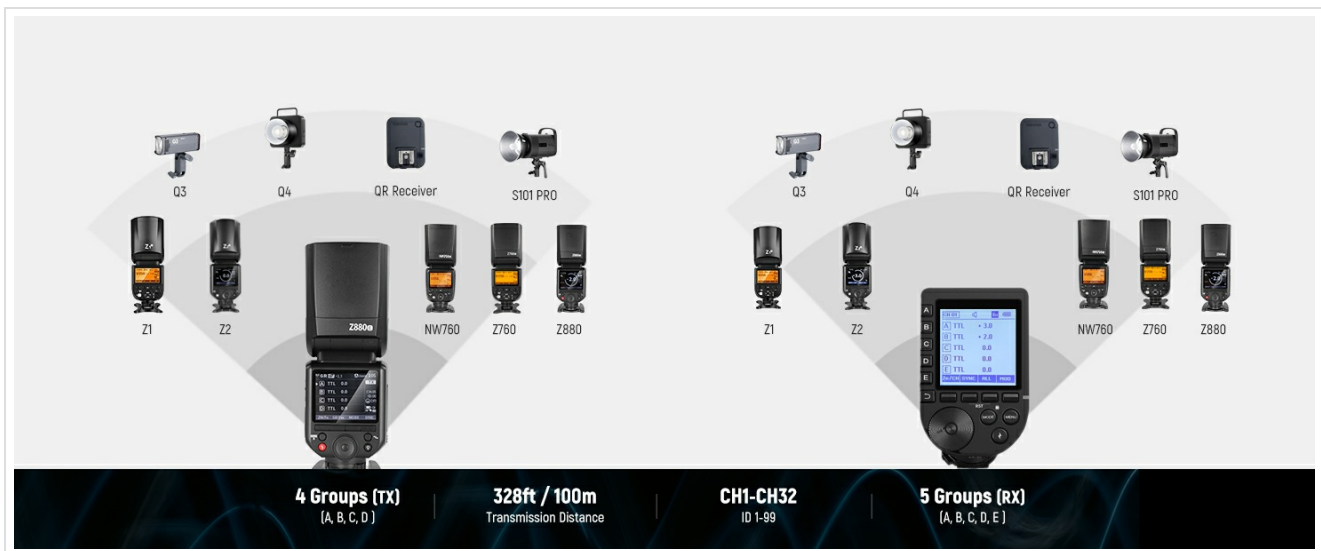
Image 4.6: Diagram illustrating the NEEWER 2.4G Wireless Q System with TX (transmitter) and RX (receiver) modes, showing compatibility with various NEEWER flash units.
