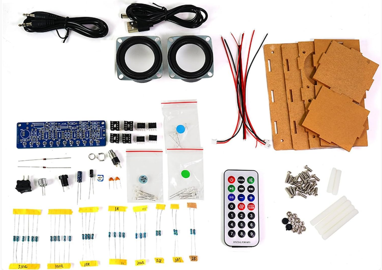
Figure 2: All individual components of the kit, including the circuit board, speakers, wires, resistors, capacitors, acrylic panels, screws, and the remote control, laid out on a surface.
