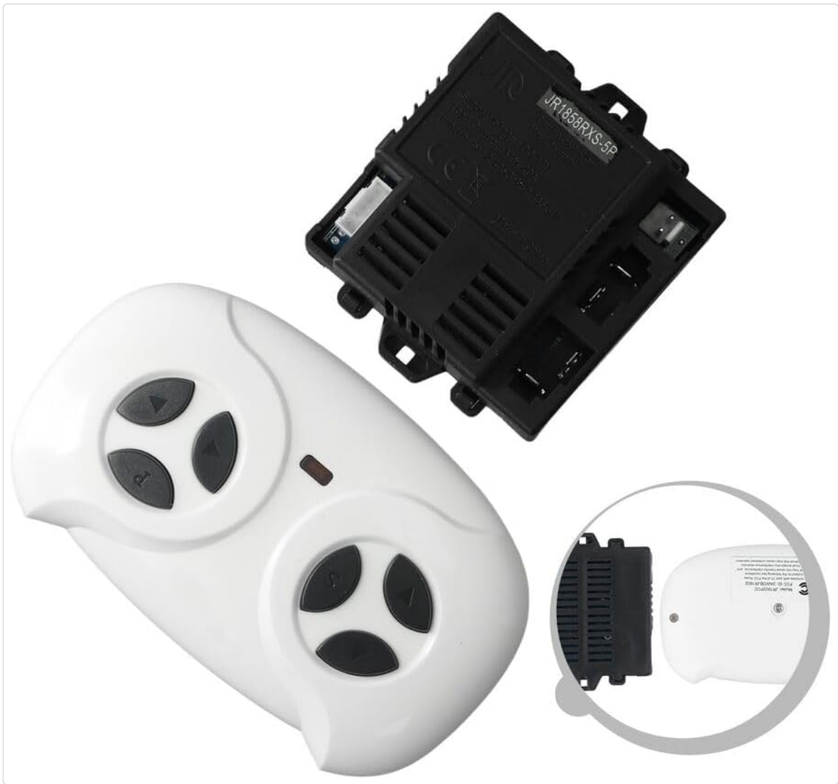
Image 2.1: Overview of the mainly JR-RX-12V Receiver and its compatible remote control.
