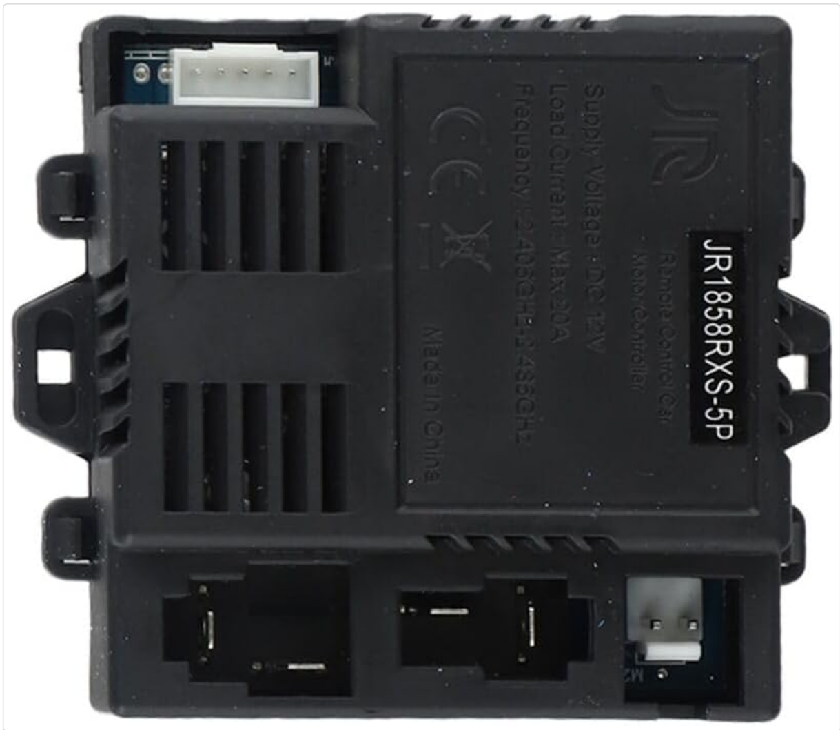
Image 2.2: Detailed view of the JR-RX-12V Receiver, showing connection ports and model number JR1858RXS-5P.
