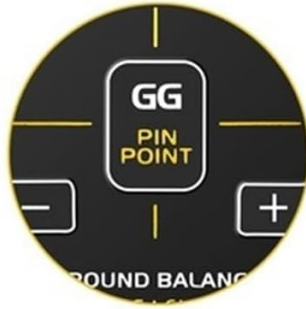
Pinpoint Searching Mode (Pinpoint button for accurate detecting)
