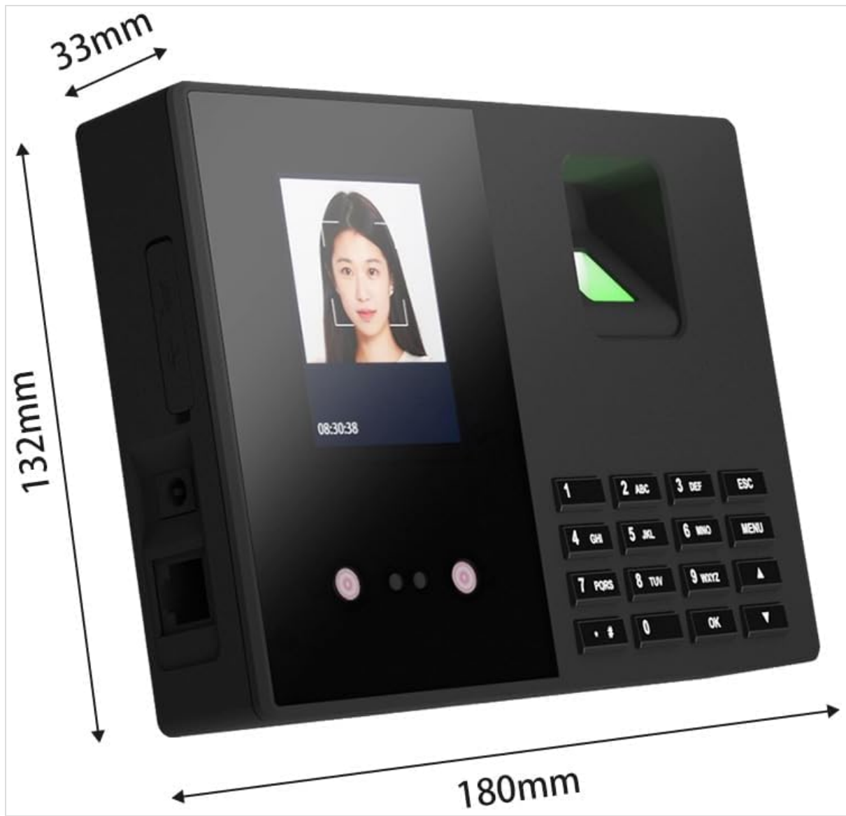
Image: Side view of the BISOFICE T200, illustrating its dimensions: 180mm length, 132mm height, and 33mm thickness.
