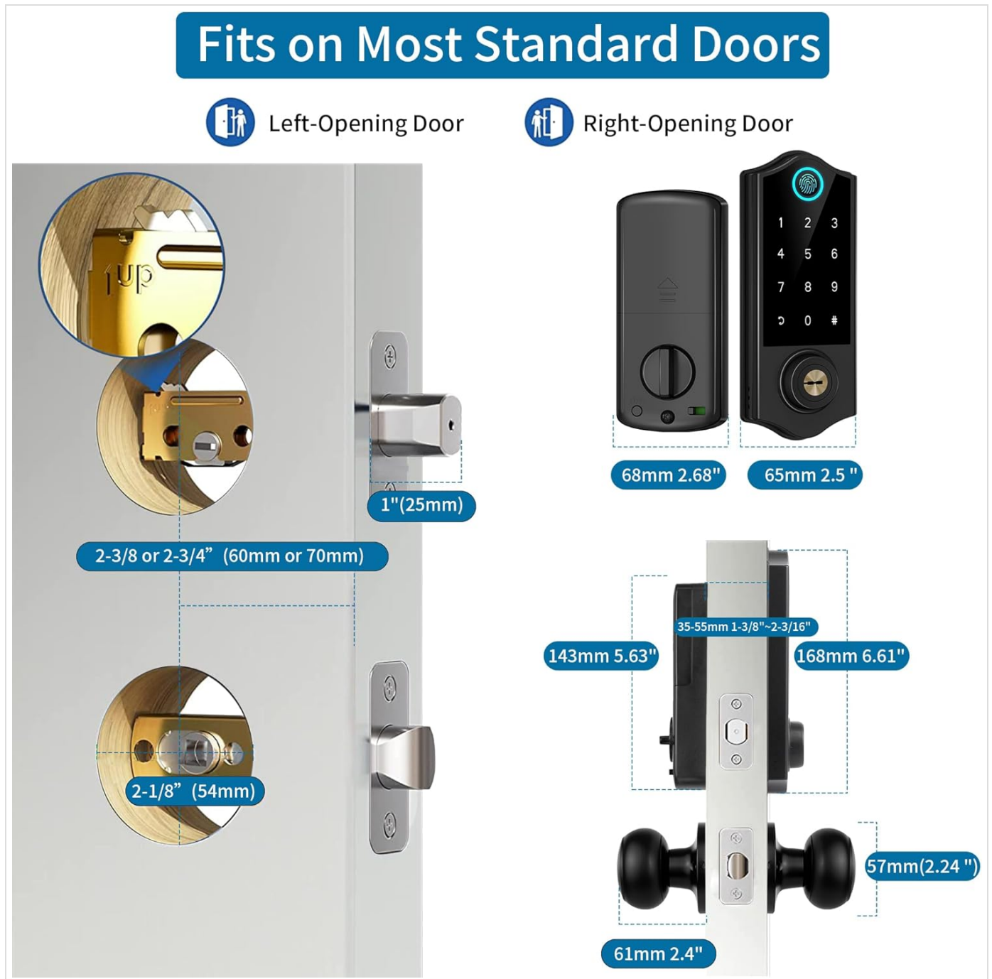
Figure 4.1: Door Compatibility and Dimensions. This image illustrates the required door measurements for proper installation, including boreholes and thickness for both left and right-opening doors.
