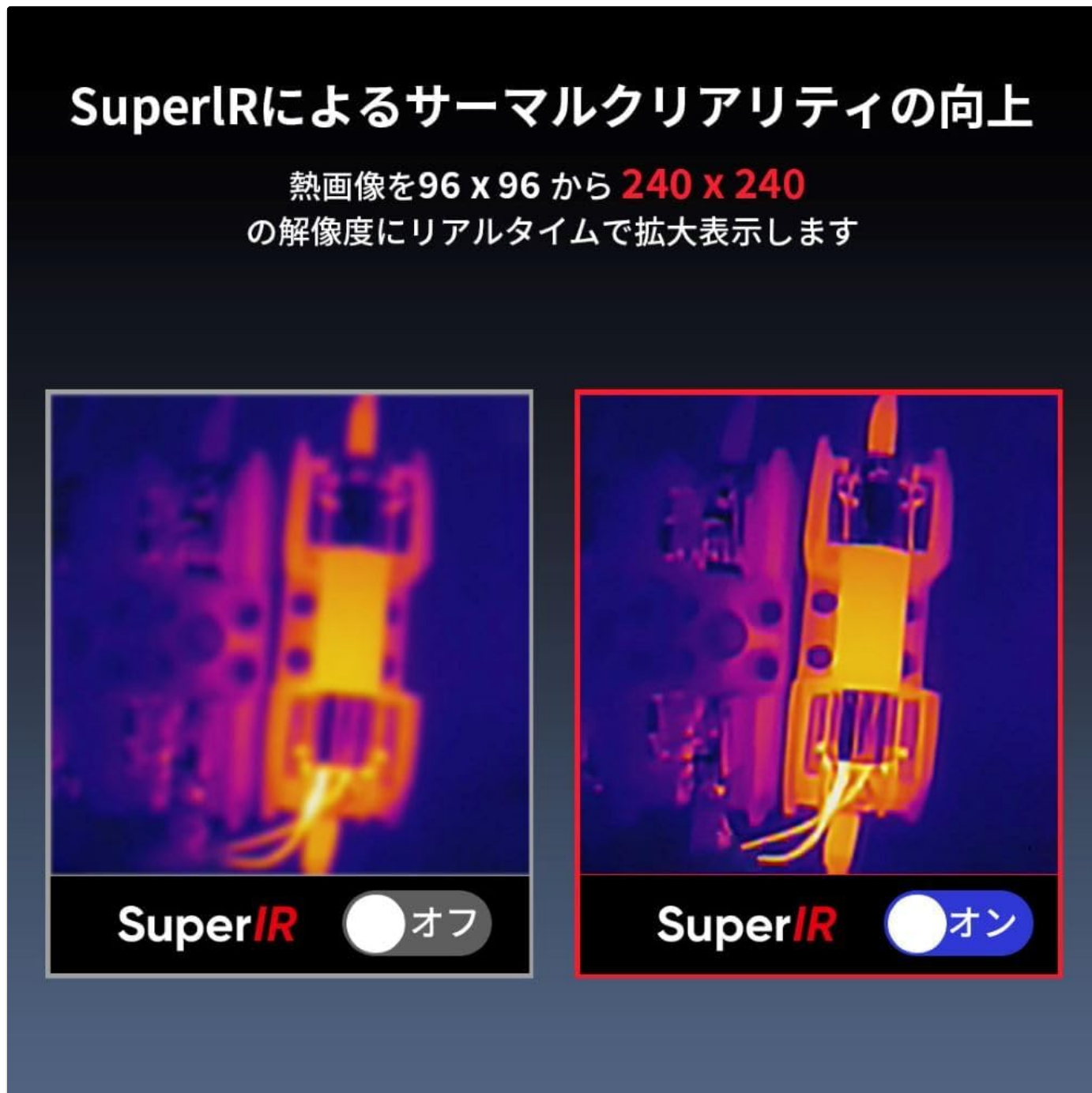
Figure 3: This image demonstrates the effectiveness of SuperIR technology. On the left, a thermal image is shown with SuperIR off (96x96 resolution). On the right, the same image with SuperIR on, displaying significantly improved clarity and detail at 240x240 resolution.
