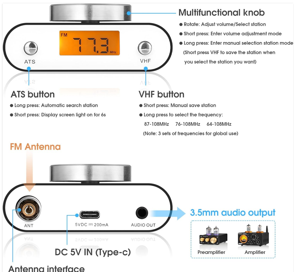
Figure 3.2: Detailed diagram illustrating the front and rear panels of the Nobsound Mini FM Radio, highlighting the multifunctional knob, ATS button, VHF button, FM antenna input, DC 5V Type-C power input, and 3.5mm audio output.
