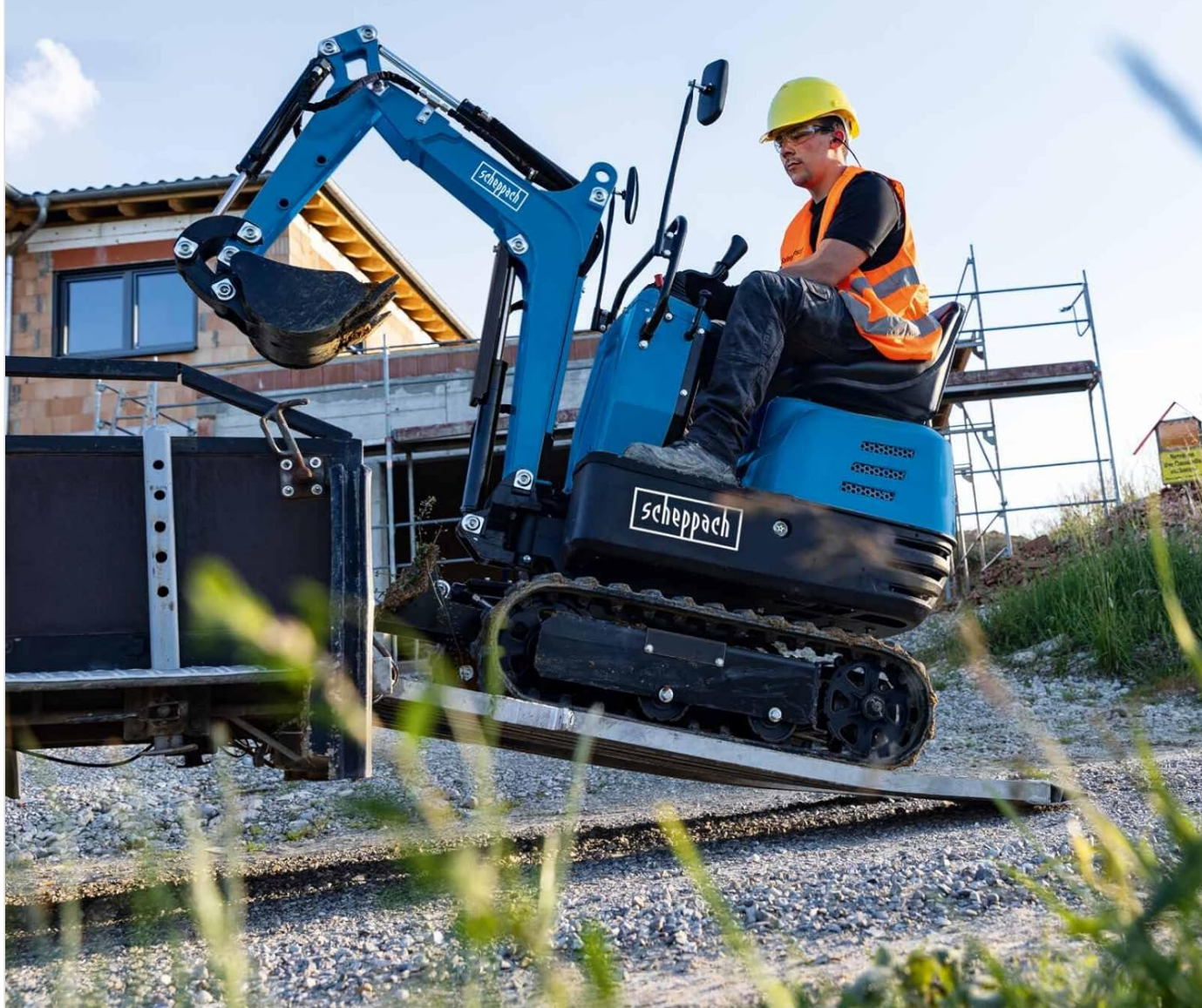
Figure 2: The excavator demonstrating its maximum climbing capacity of 15 degrees. Always operate on stable ground and be mindful of slopes.
