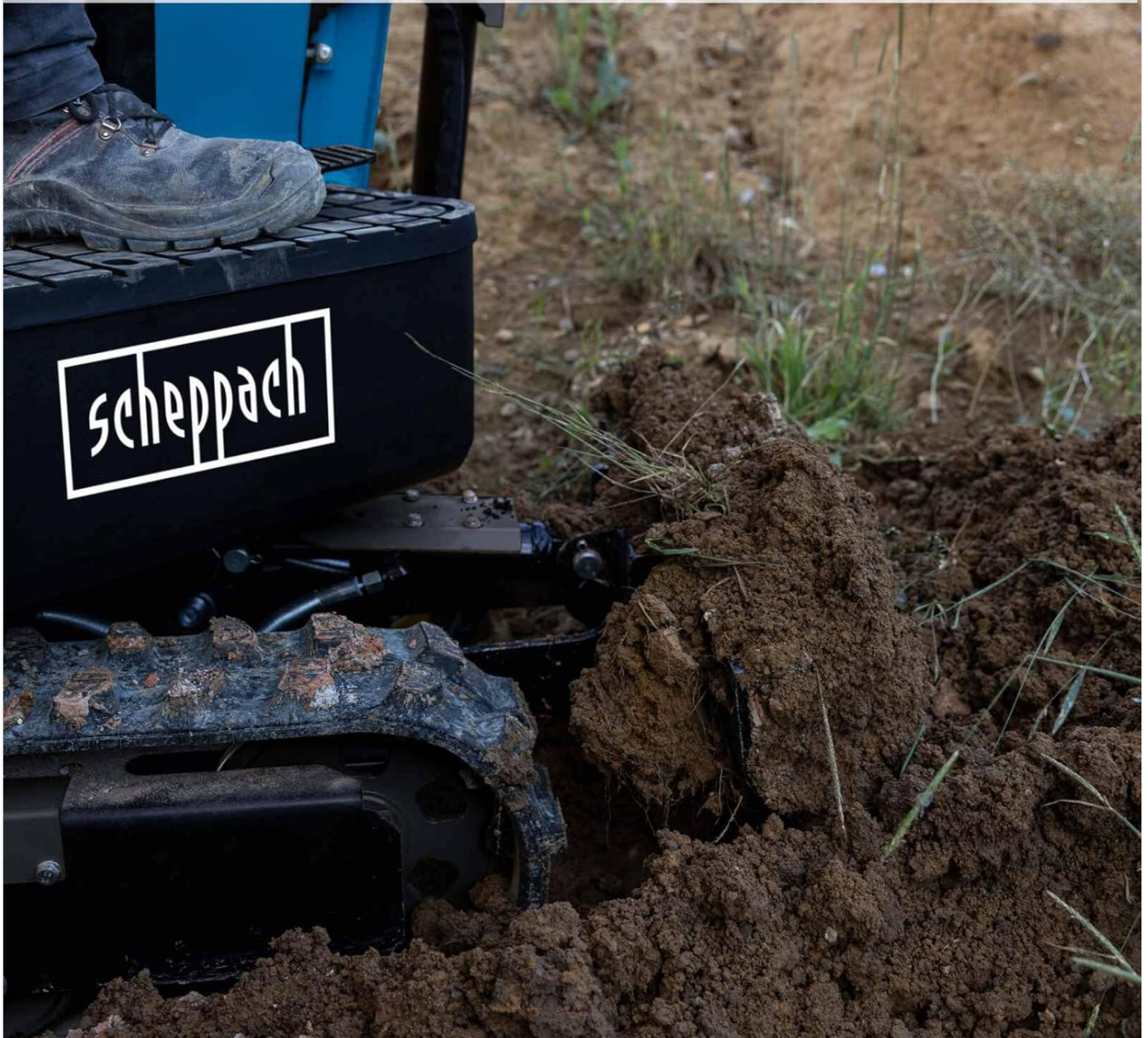
Figure 8: The large, lowerable leveling blade in action, used for stabilizing the boom or leveling the ground.
