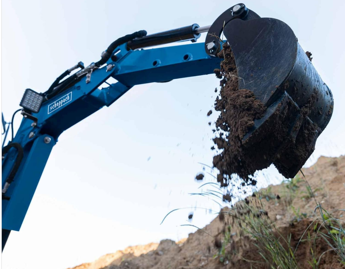
Figure 7: Close-up of the excavator bucket, showing its 0.011 m 3 volume and 290 mm width, suitable for efficient material handling.
