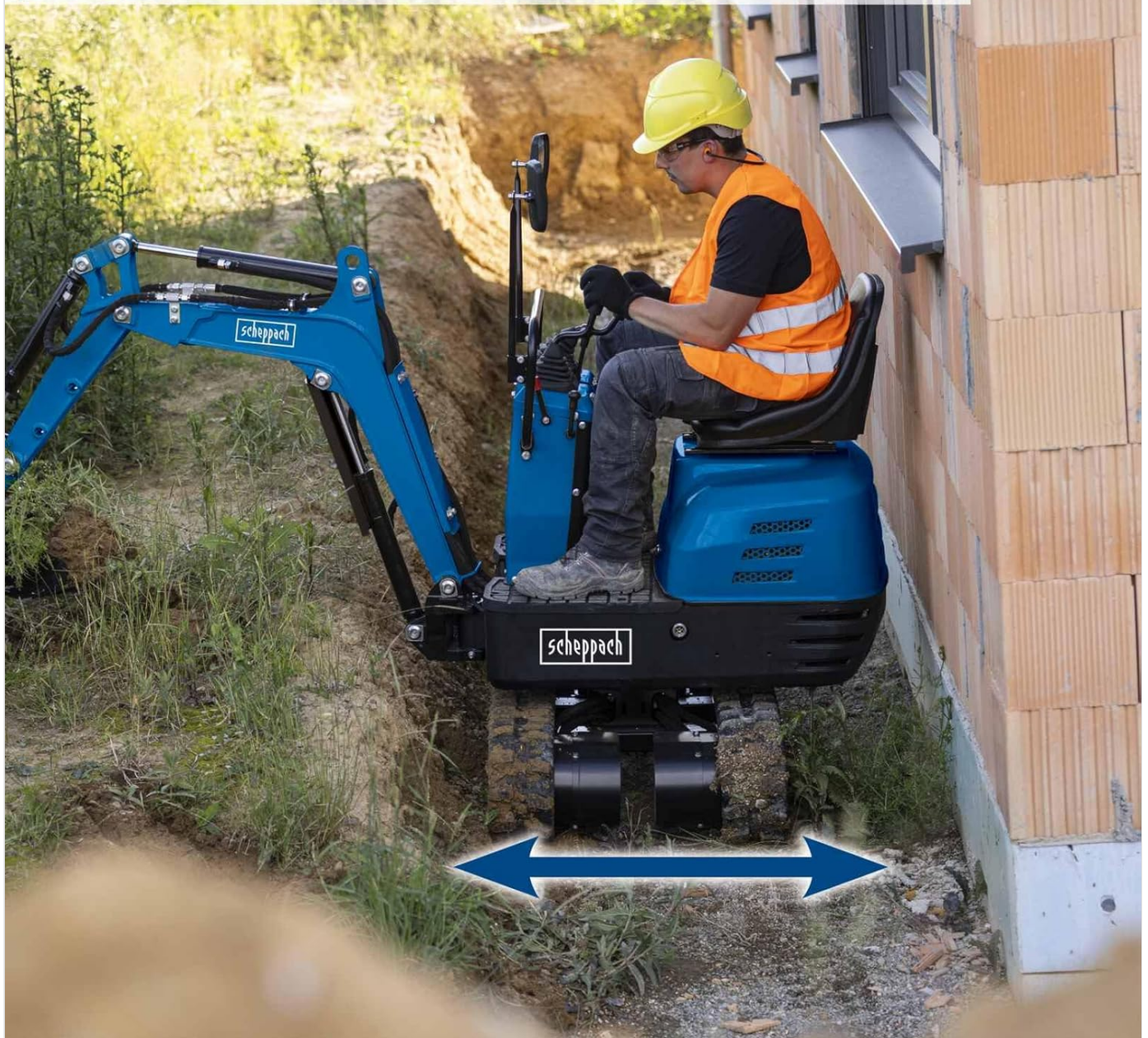
Figure 4: The excavator operating in a narrow passage, demonstrating its 690 mm track width, which is ideal for confined spaces.
