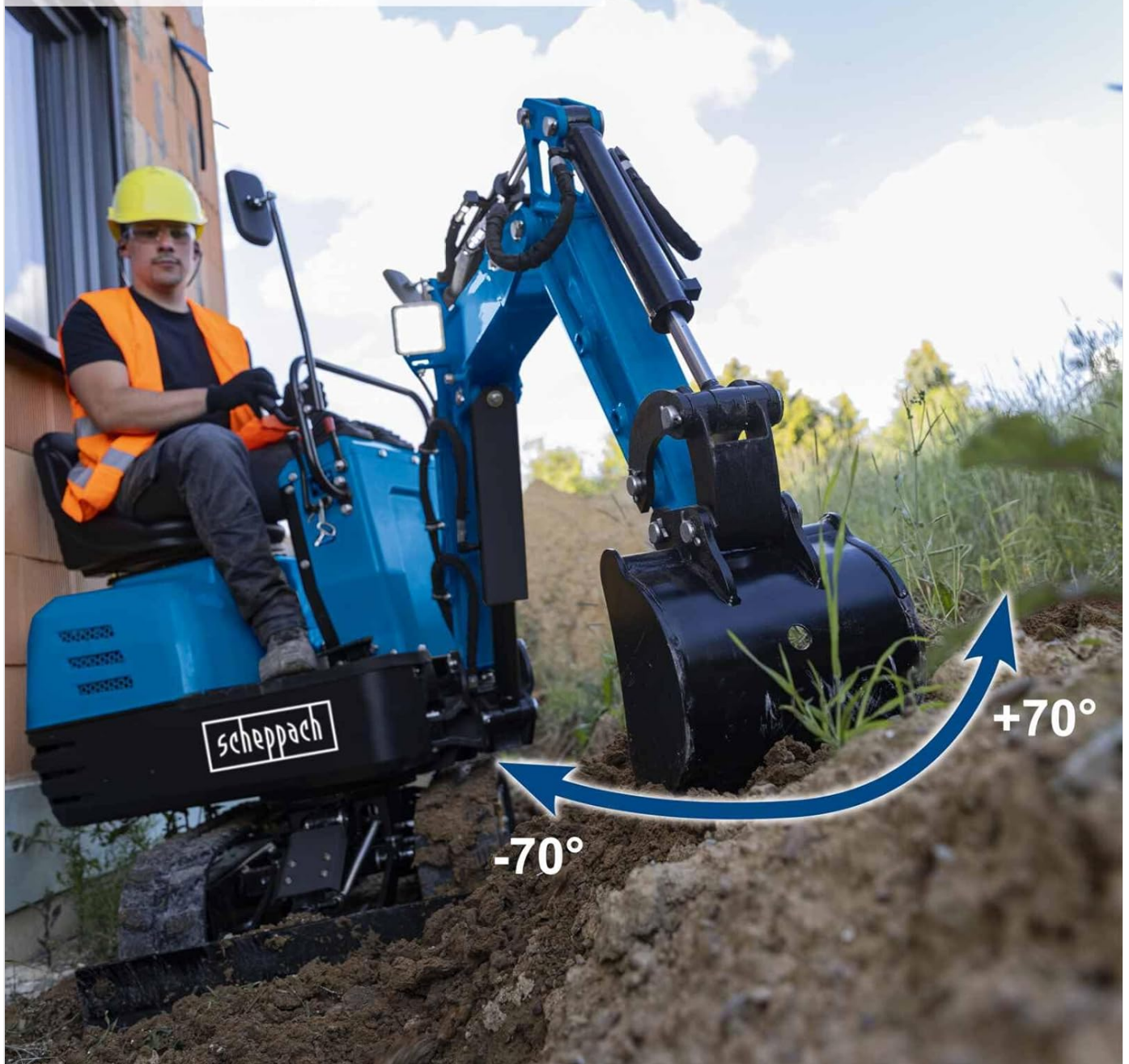
Figure 6: Illustrates the boom's pivot range of \pm 70 degrees, providing flexibility for various digging tasks.
