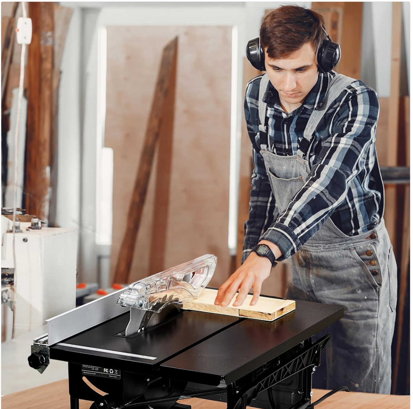
Figure 4.1: Blade guard (monocular shield) properly installed.
