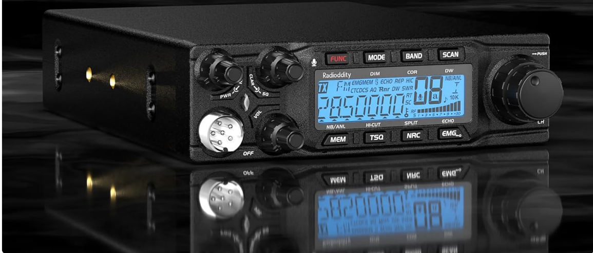
Figure 4: Illustration of the multi-modulation capabilities of the QT80.
