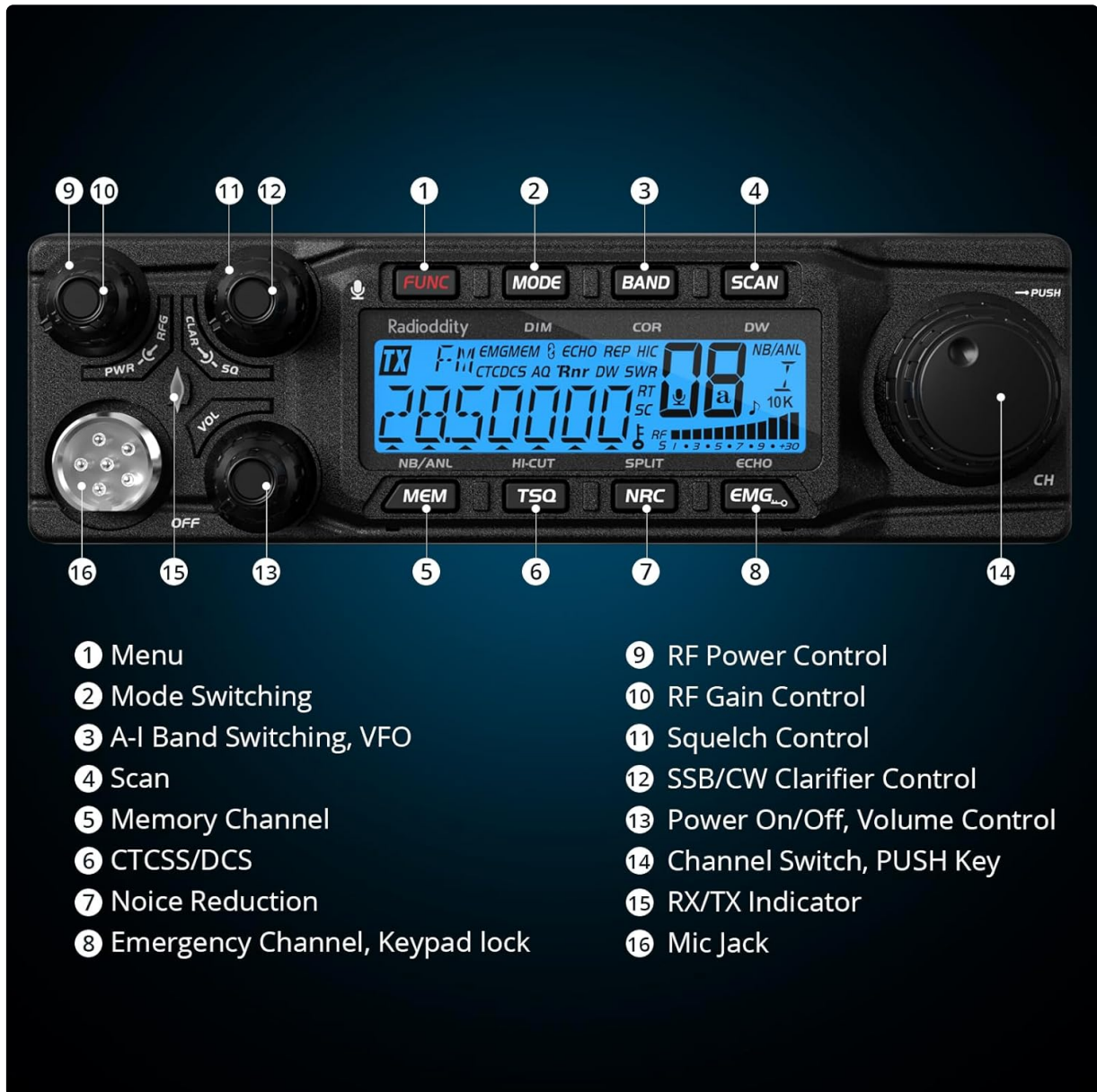
Figure 8: Detailed diagram of the QT80's front panel controls and their corresponding functions.
