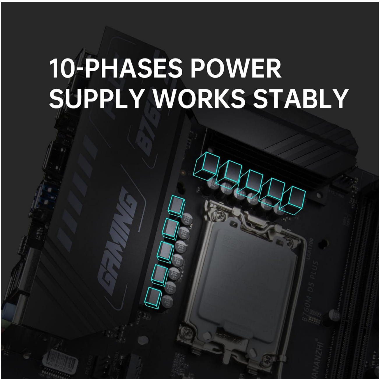
Image: A close-up of the motherboard's CPU power delivery area, illustrating the 10-phase power supply components.
