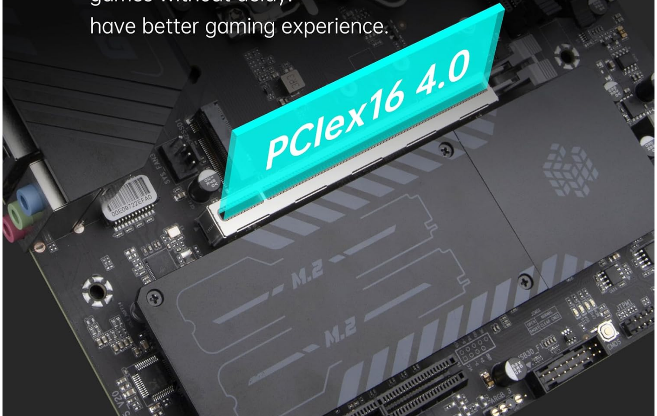
Image: The PCIe x16 4.0 slot is highlighted on the motherboard, indicating its high-speed data transfer capability for graphics cards.
