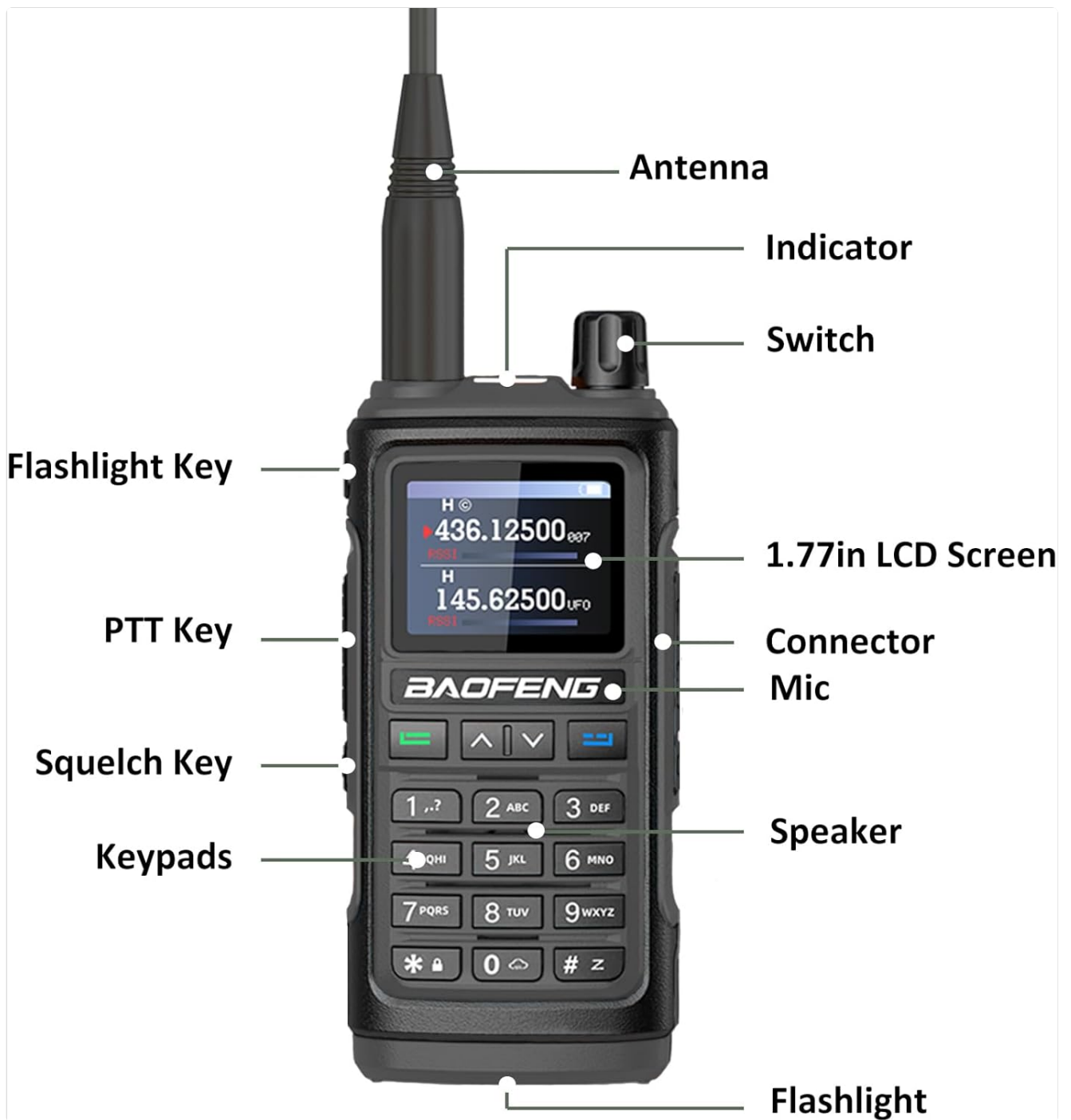
Figure 2: Front and side view of the UV-17H radio with key components labeled, including the antenna, indicator light, power switch, flashlight key, Push-to-Talk (PTT) button, squelch key, numeric keypads, 1.77-inch LCD screen, microphone connector, speaker, and bottom flashlight.
