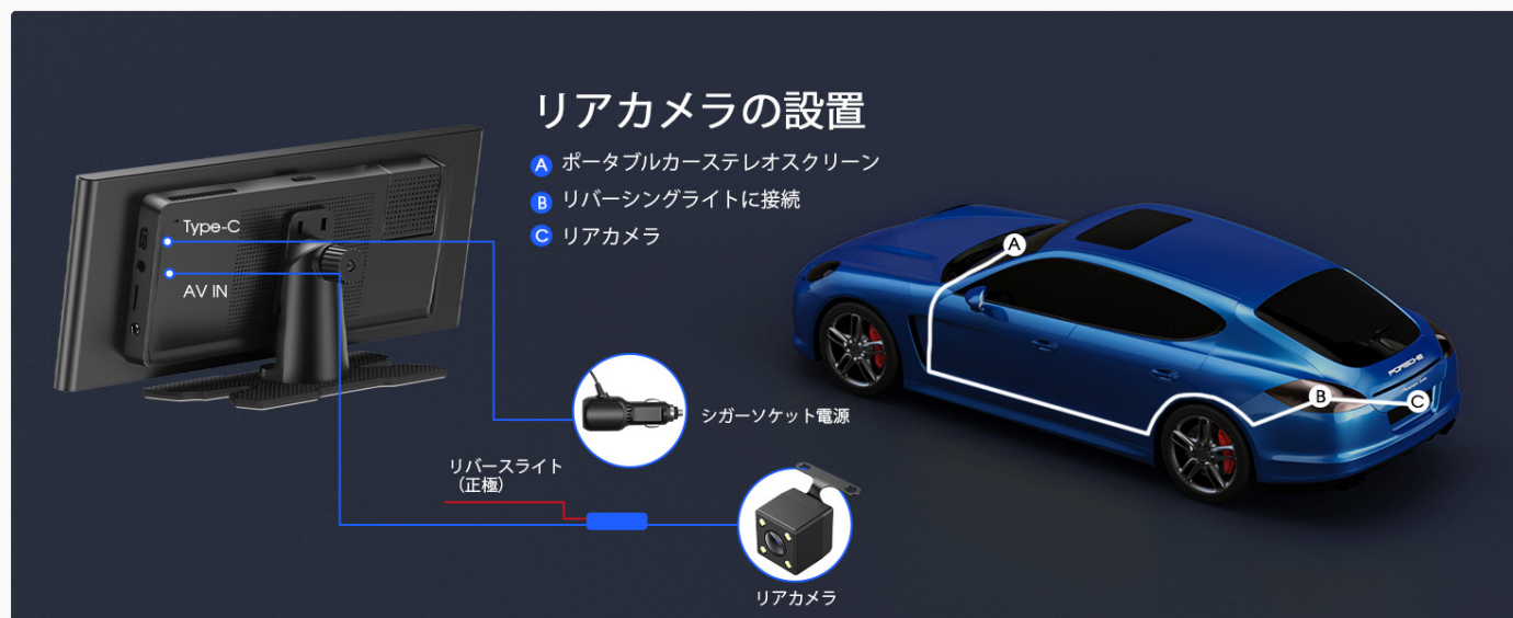
Rear camera wiring diagram, showing connections to the display and vehicle's reverse light.
