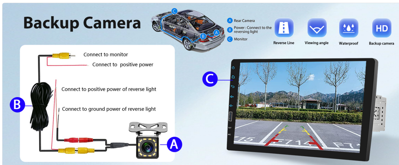
Image: Diagram showing the connections for the backup camera, including video signal to the head unit and power connections to the reverse light circuit.
