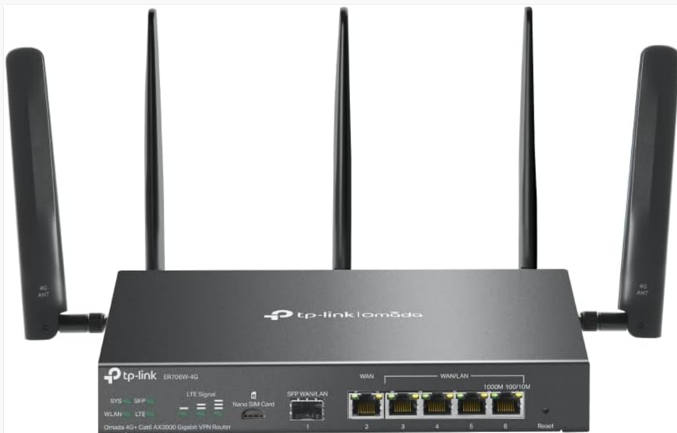
Image: Front view of the TP-Link ER706W-4G Omada VPN Gateway Router, showing the status LEDs, SIM card slot, WAN/LAN ports, and detachable antennas.
