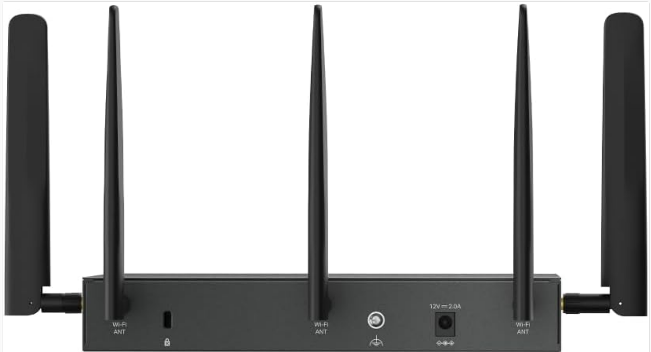
Image: Rear view of the ER706W-4G, showing the Wi-Fi antenna connectors, power input, and grounding terminal.
