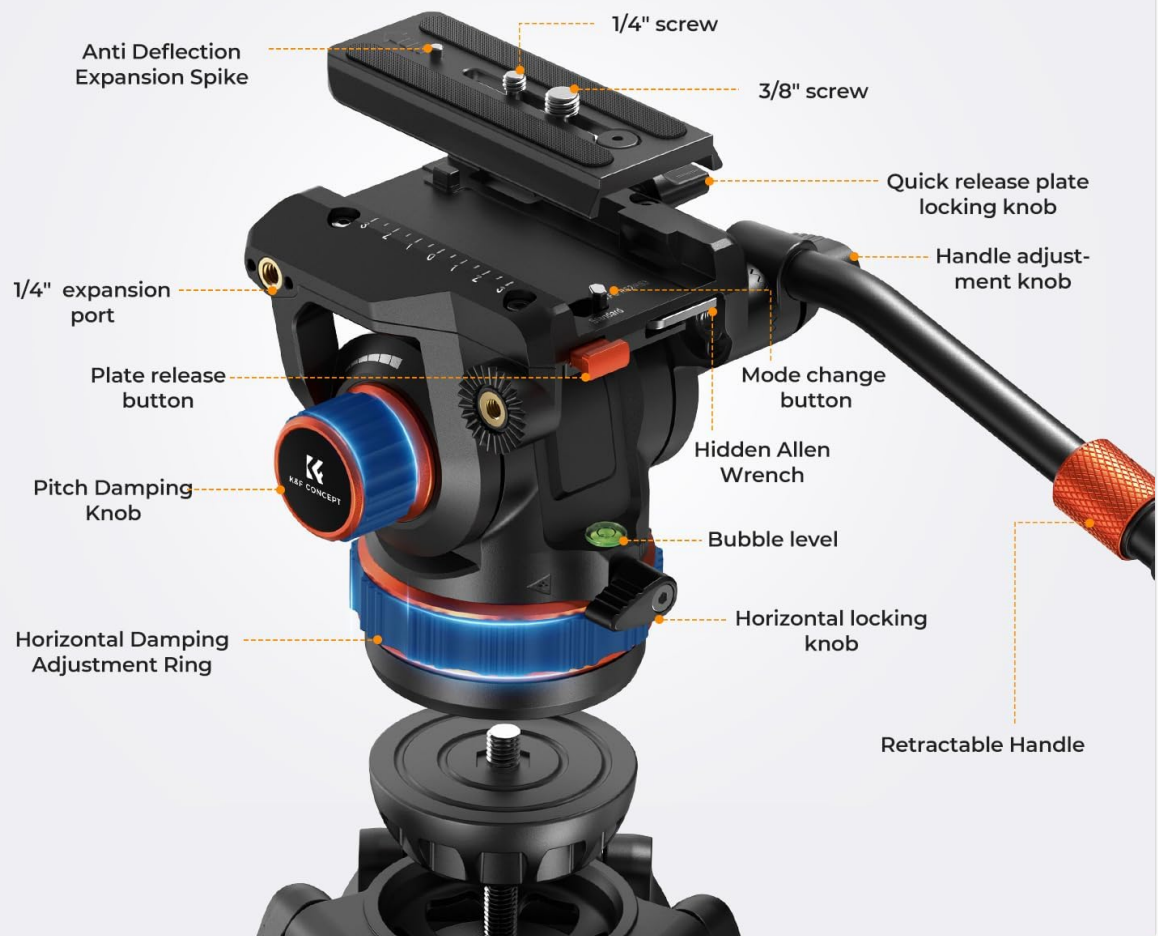
Figure 1: Professional Fluid Head Components
