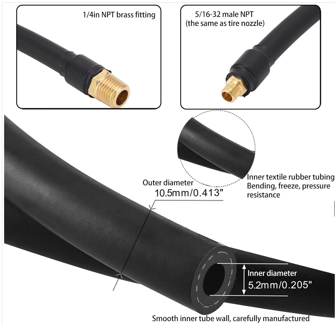
Image 3.2: Detailed view of the air compressor hose, highlighting the 1/4in NPT brass fitting, the 5/16-32 male NPT fitting (tire nozzle compatible), and measurements for the outer diameter (10.5mm/0.413in) and inner diameter (5.2mm/0.205in).
