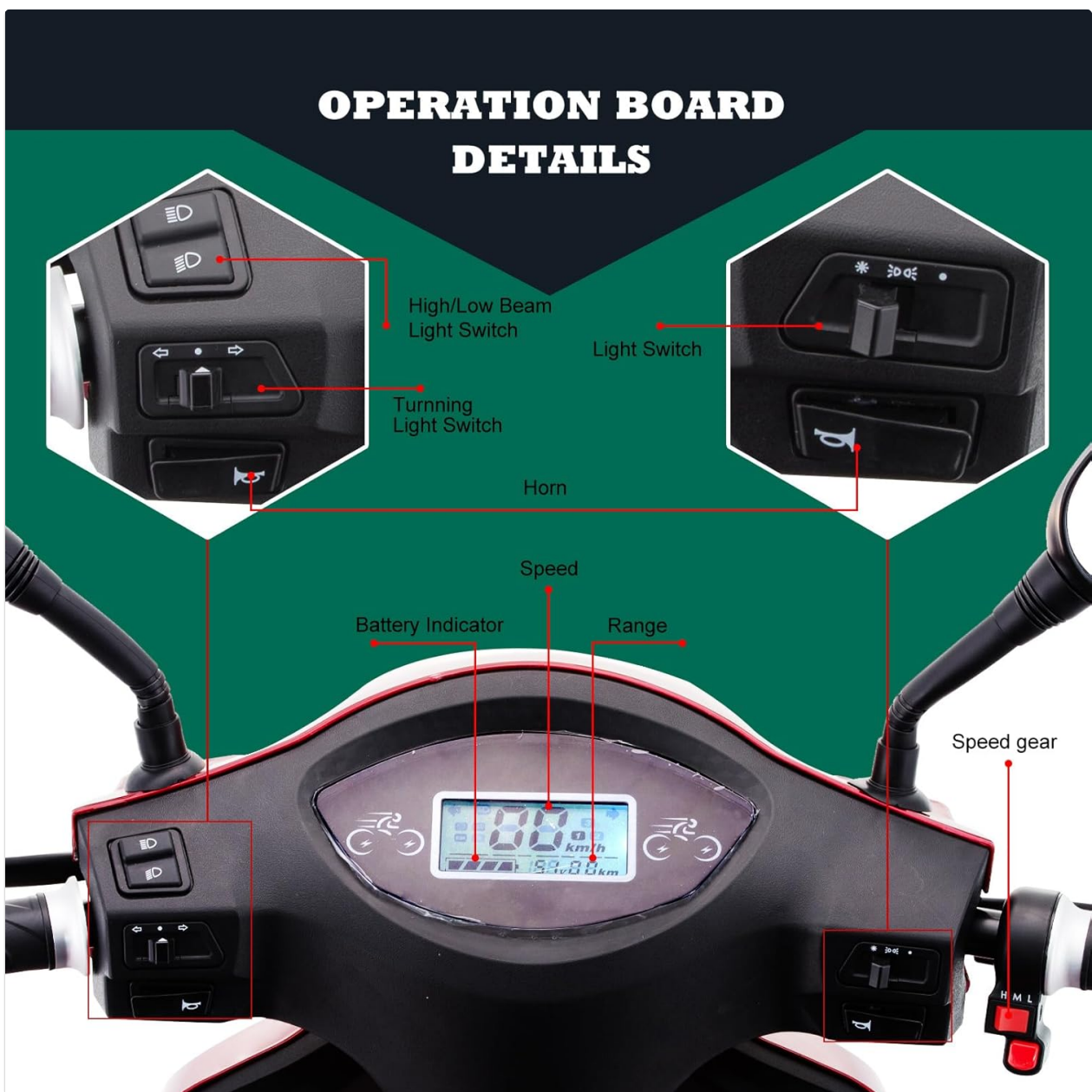
Figure 2: Operation Board Details
