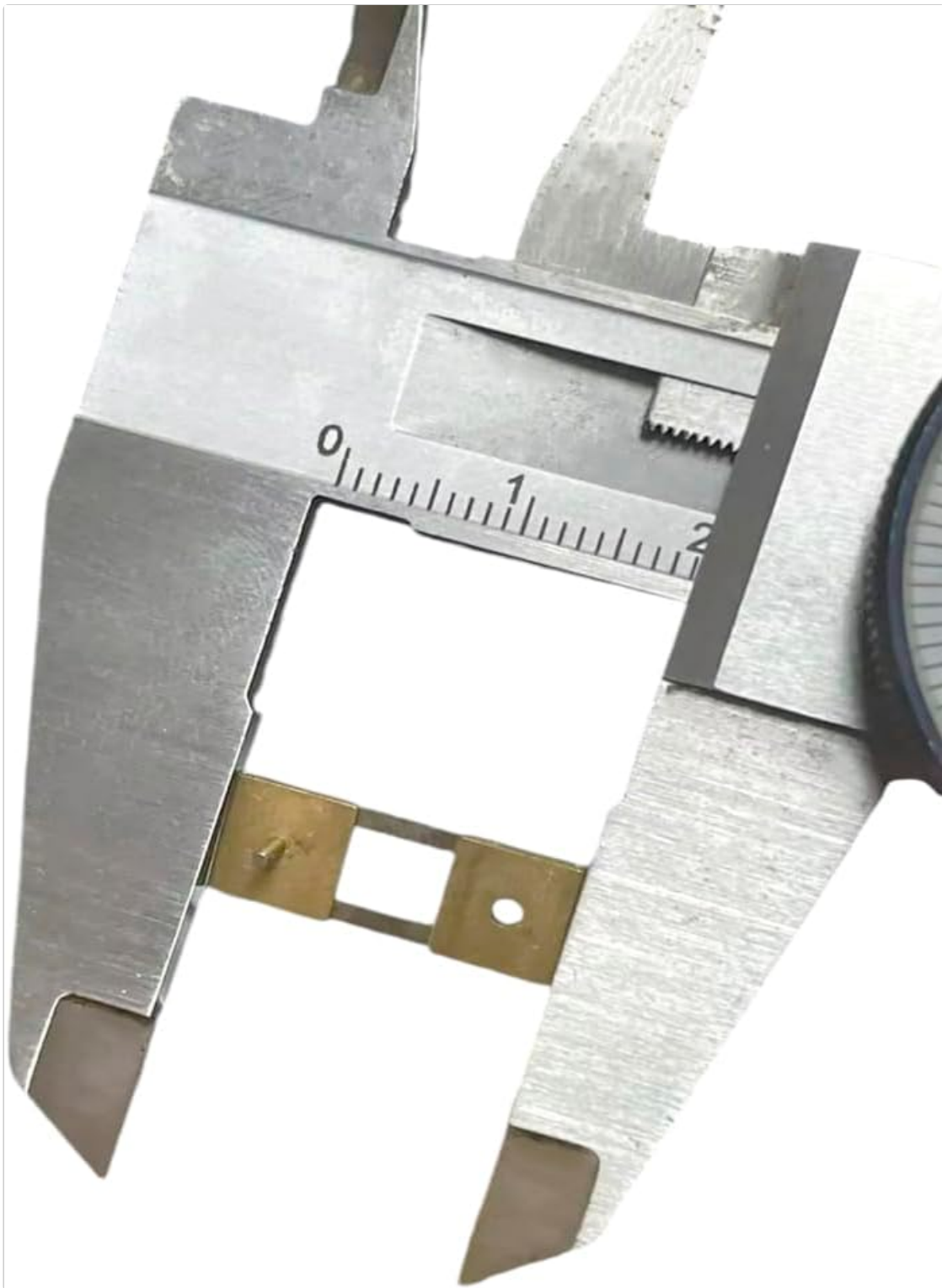
Image 3.3: A suspension spring held by a digital caliper, demonstrating its width measurement.
