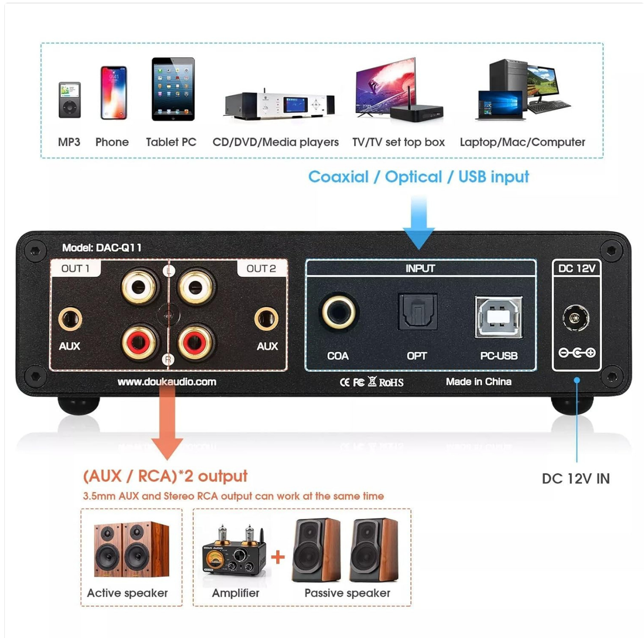
Figure 7: Rear panel connection diagram for the Douk Audio Q11.
