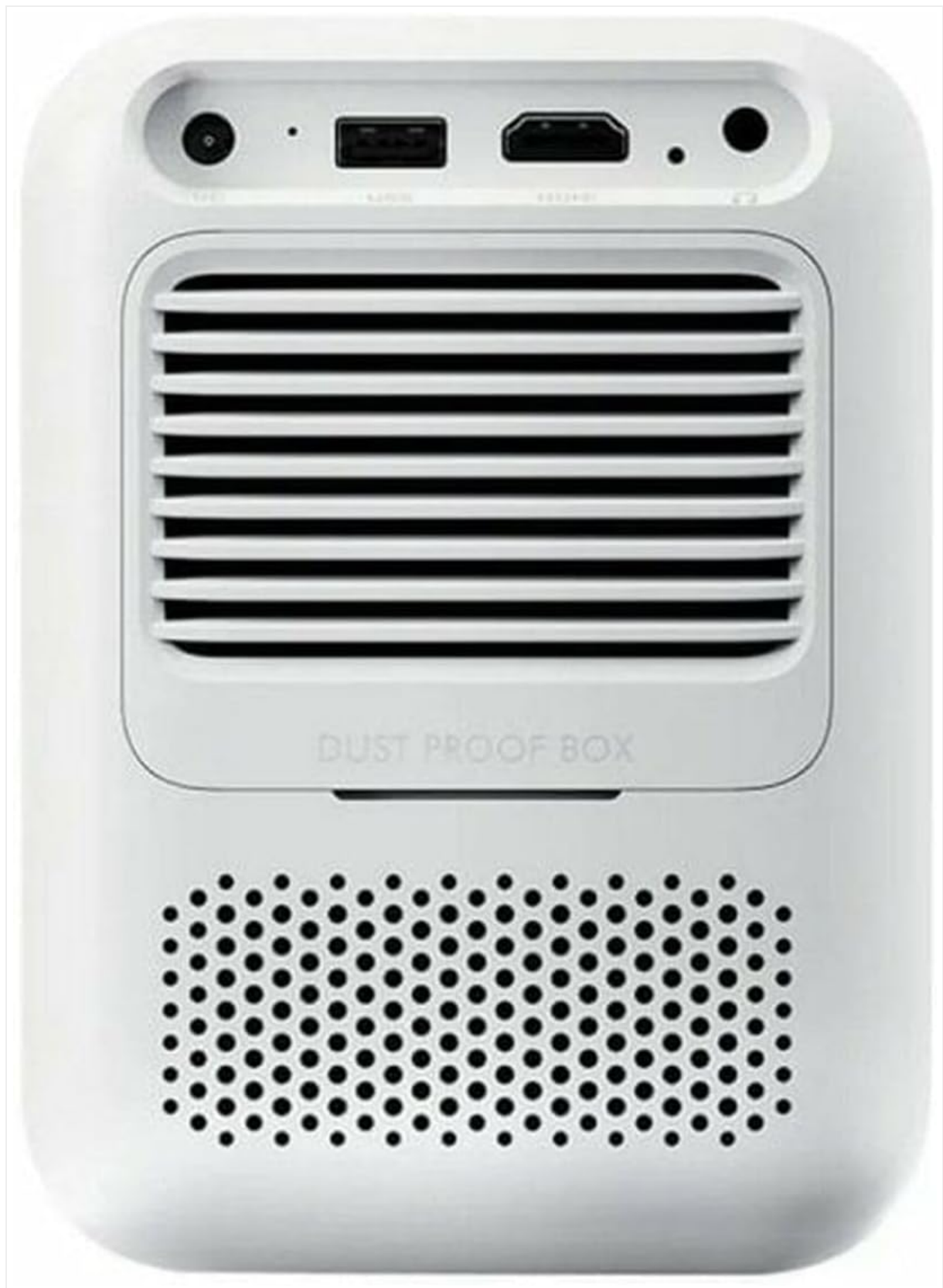
Figure 2: Rear view of the WANBO DALI 1 Projector, displaying the power input, USB port, HDMI port, and audio jack.
