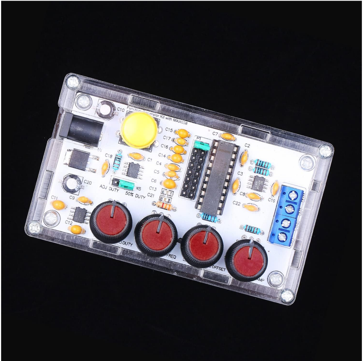
Image: Top view of the assembled MAX038, highlighting the four main control knobs for frequency, duty cycle, offset, and amplitude, along with waveform selection switches.
