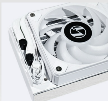
the fan cables are integrated into the cooling tubes, simplifying the connection process.
