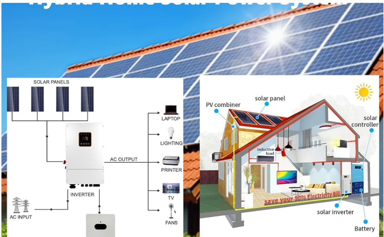
Figure 5: Simplified diagram illustrating the connections within a hybrid home solar power system.
