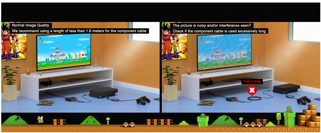
Image: A side-by-side comparison showing "Normal Image Quality" with a short component cable (less than 1.8m) and a "Noisy Image Quality" with an excessively long component cable, illustrating the impact of cable length on signal integrity.
