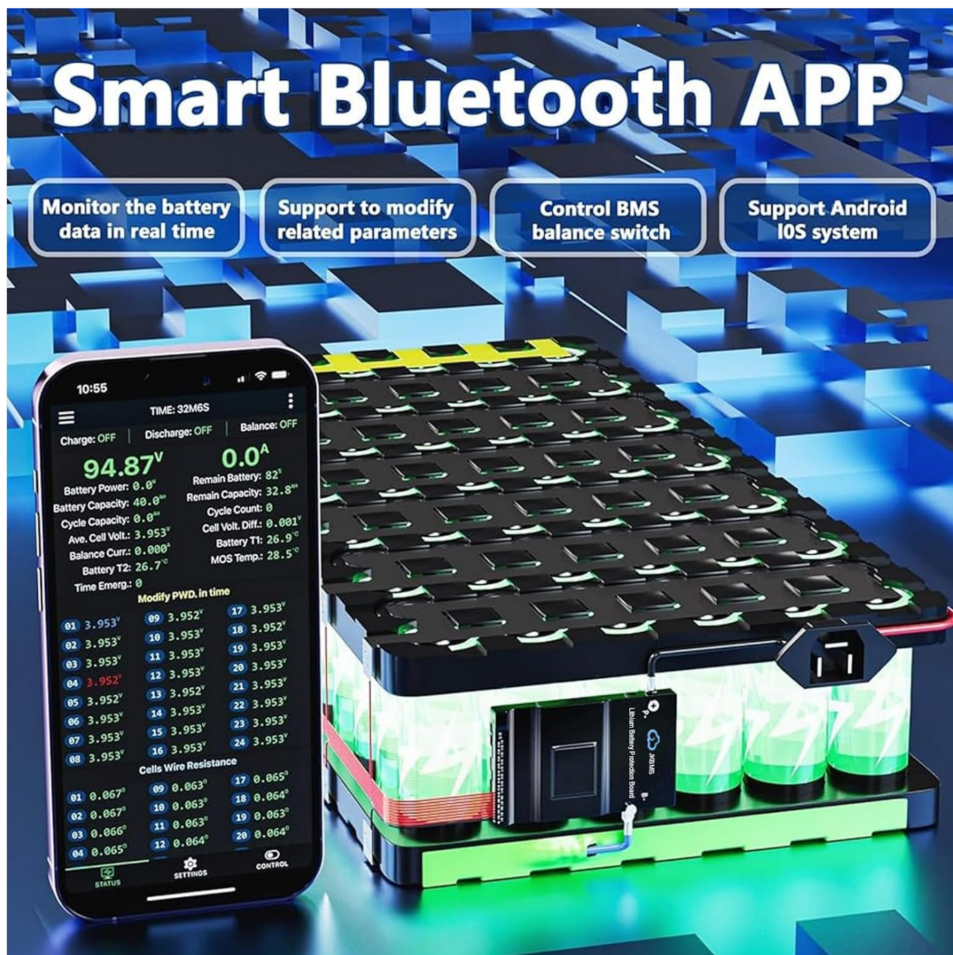
Image 6: Screenshot of the Smart Bluetooth App interface. This image shows the mobile application displaying real-time battery data, including voltage, current, temperature, and individual cell readings, demonstrating the monitoring capabilities.
