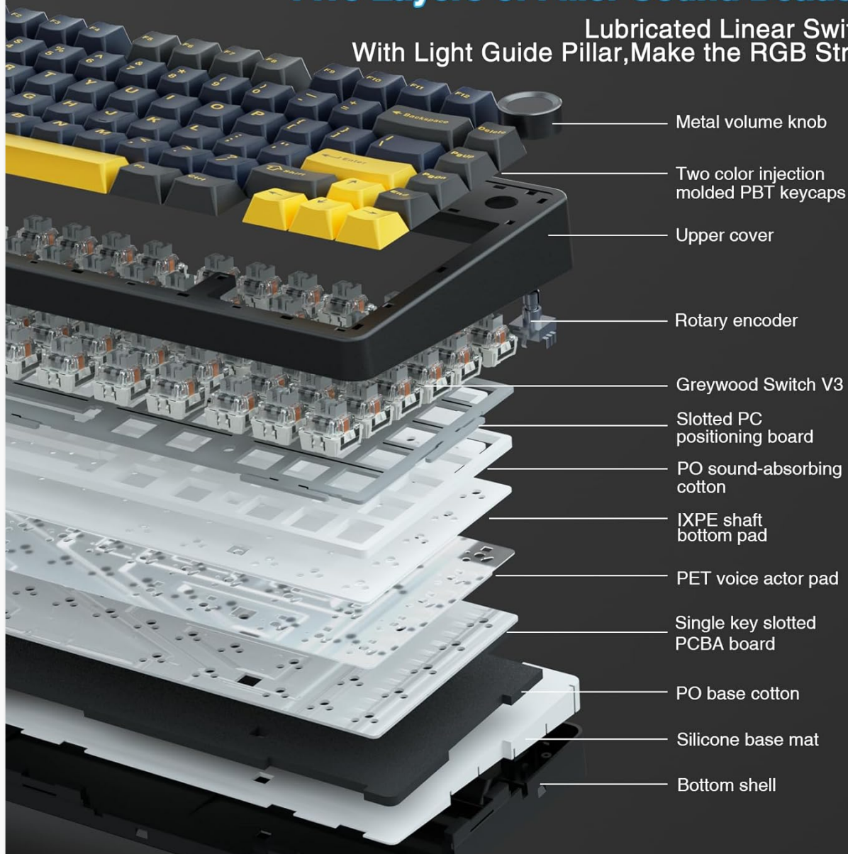
Image 3.4: Diagram illustrating the advanced gasket structural design and five layers of sound dampening in the AULA F75 keyboard.
