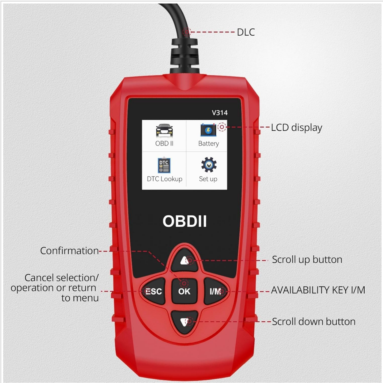
Image 2.1: Labeled diagram of the BINTA OBD2 Scanner V314, highlighting its components and control buttons.
