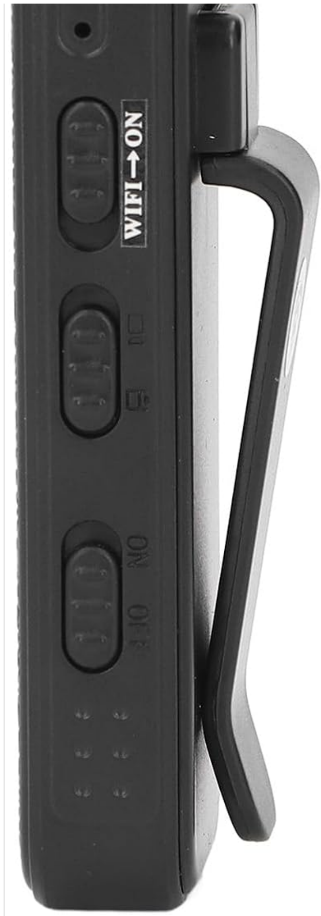
Figure 2.2: Side view of the Yoidesu Body Camera with labeled controls including Night Vision ON/OFF, WiFi ON/OFF, Video/Save, ON/OFF, Reset button, and TF-Card slot.
