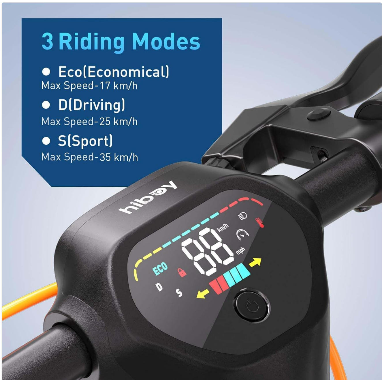
Image: The scooter's digital display indicating the three riding modes: Eco, D (Driving), and S (Sport).
