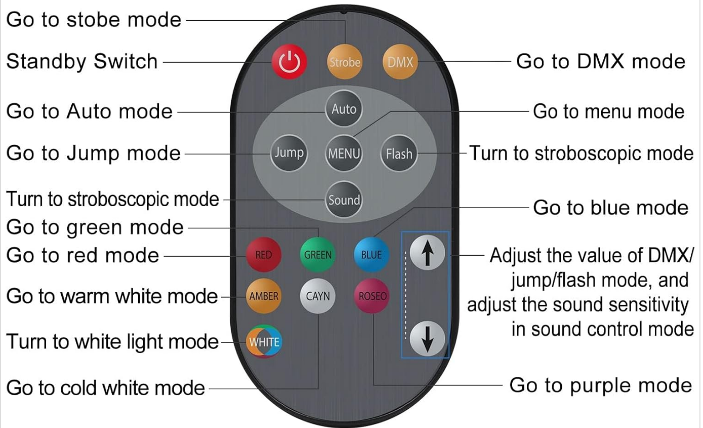
Figure 5.1: Remote Control Layout and Functions
