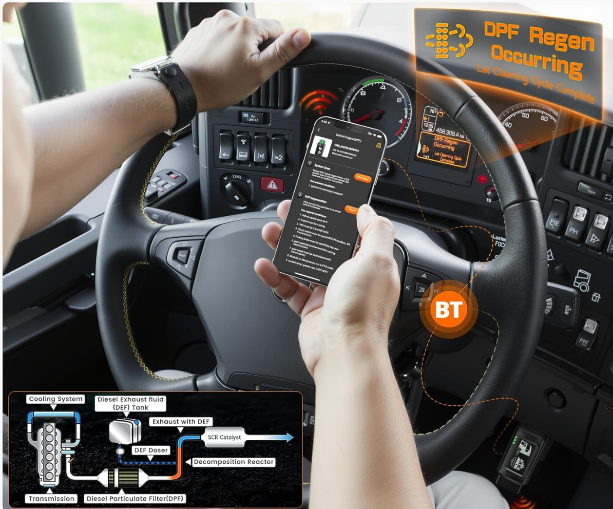
Image: A smartphone displaying "DPF Regen Occurring" while connected to the ANCEL HD110 scanner, illustrating the DPF regeneration process.
