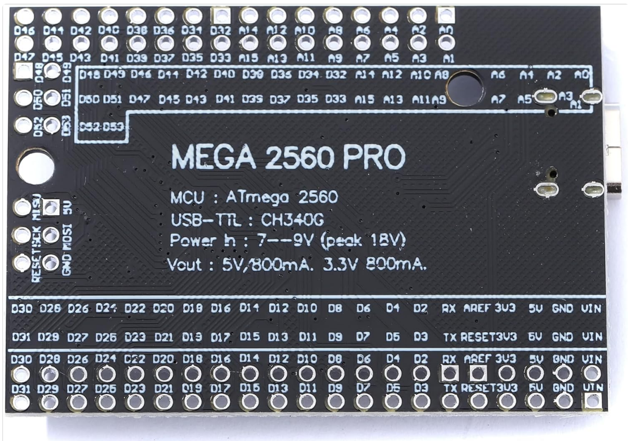
Image: Bottom view of the Teyleten Robot MEGA2560 PRO Embed Module, displaying key specifications and pin labels.
