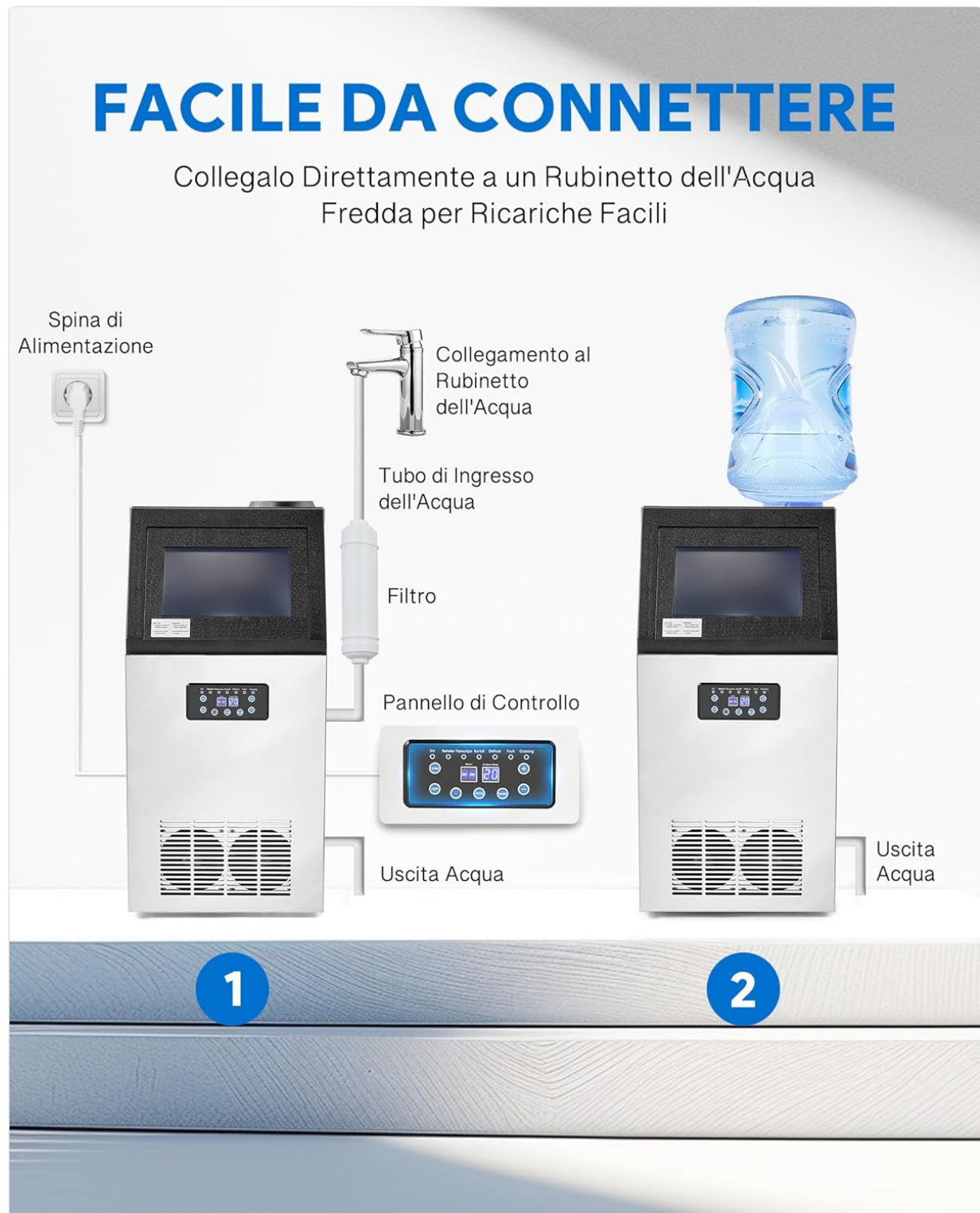
Image 5.1: Easy Water Connection. This diagram illustrates the two primary methods for connecting the ice maker to a water source. Option 1 shows a direct connection to a cold water tap with an inline filter and power plug. Option 2 shows
