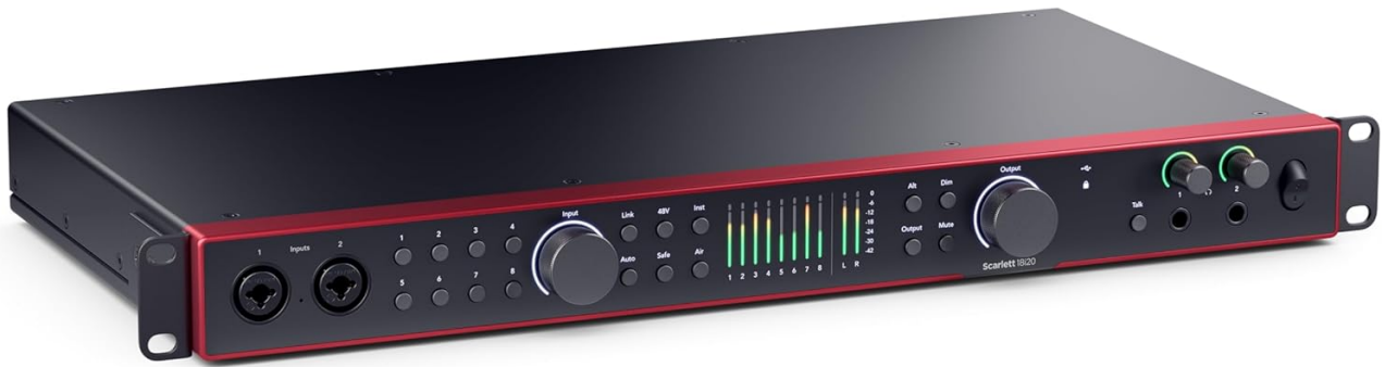
Figure 1: Front Panel Overview. This image displays the front panel of the Scarlett 18i20 4th Gen audio interface, highlighting the input jacks, gain knobs, and monitoring controls.
