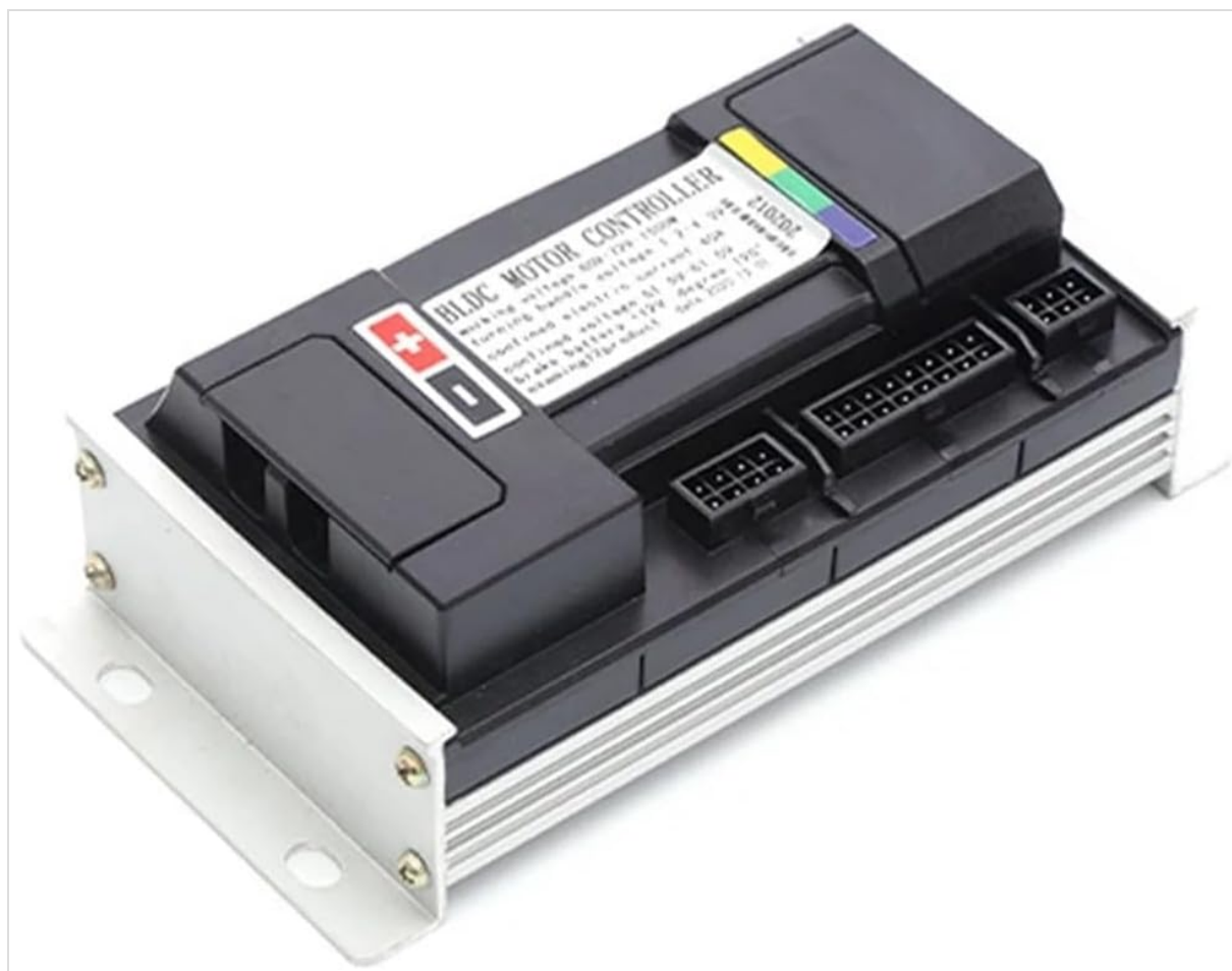
Figure 3.2: A closer view of the controller's top surface, highlighting the "BLDC MOTOR CONTROLLER" label and specifications such as working voltage (48V-72V) and rated power (1500W). Various connection ports are also visible.
