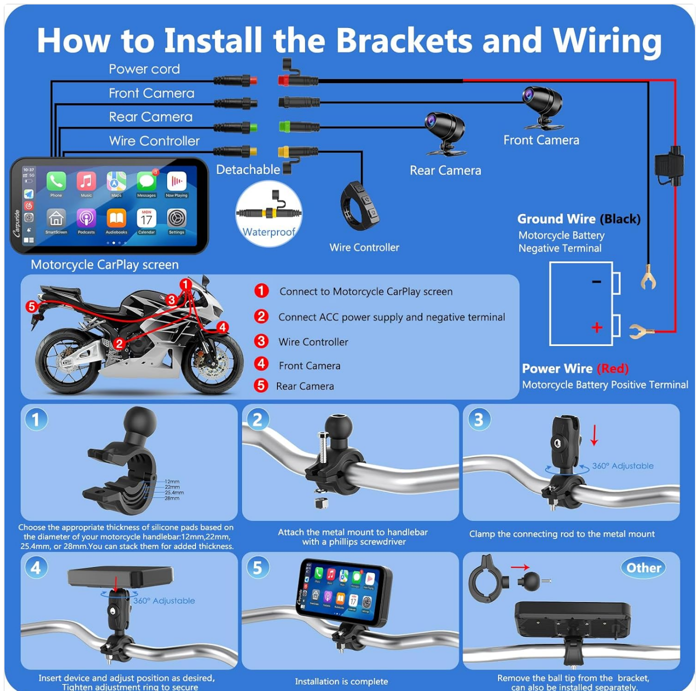
Figure 4: Detailed wiring and mounting instructions for the Carpuride W603D.
