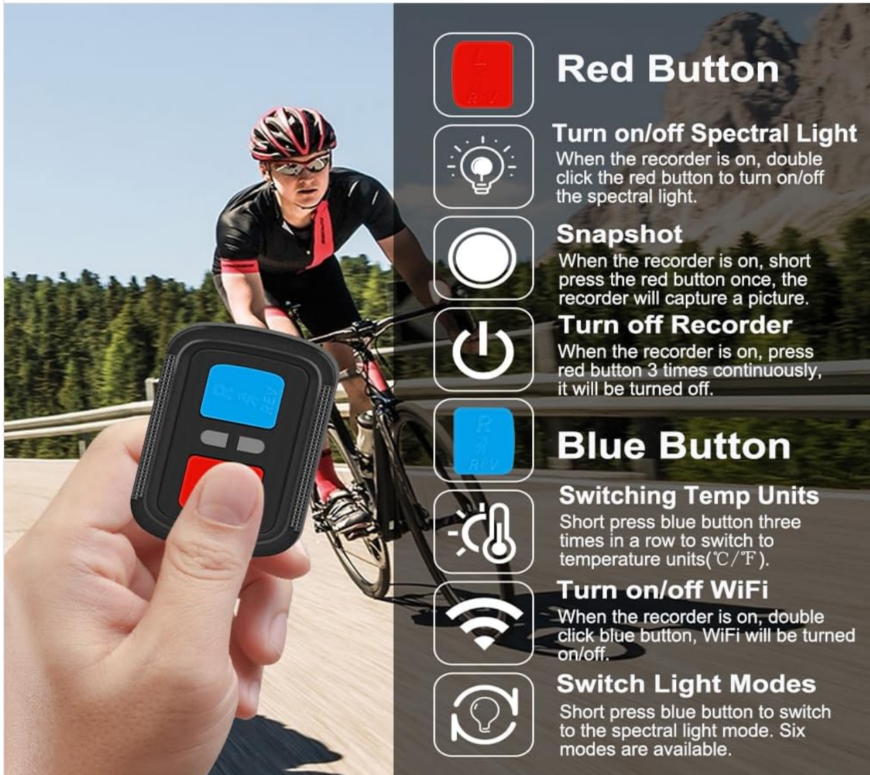
Image: A visual guide to the functions of the red and blue buttons on the wireless remote control.
