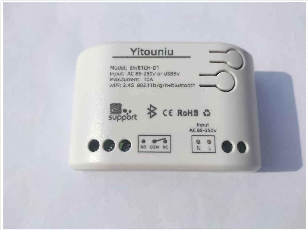
Image 3.2: Close-up view of the Yitouniu EWELink Smart WiFi Switch Relay, showing input terminals (N, L), output terminals (NO, COM, NC), and model information.
