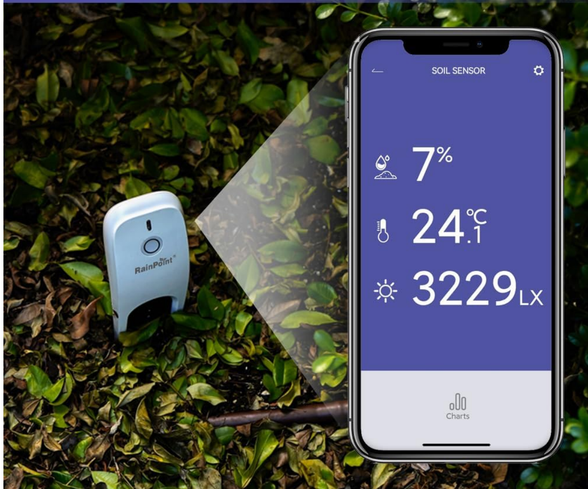
Image 4.1: The HomGar app interface showing real-time soil moisture (7%), temperature (24.1°C), and light intensity (3229 LX).
