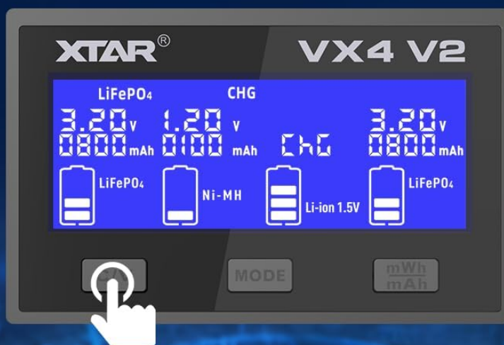
Figure 5: Switching between Standard and LiFePO4 charging modes.
