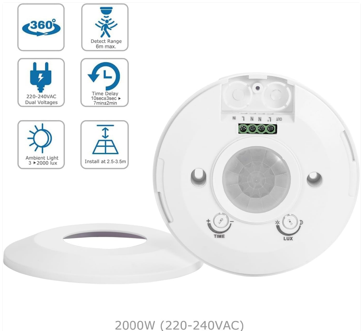
Image 1: Greluma PIR Motion Sensor Light Switch with key features highlighted. This image shows the front view of the sensor, its adjustment knobs for time and LUX, and connection terminals. Icons around it indicate 360-degree detection, 6m max range, 220-240VAC dual voltages, 10s-7min time delay, 3-2000 lux ambient light, and 2.5-3.5m installation height.
