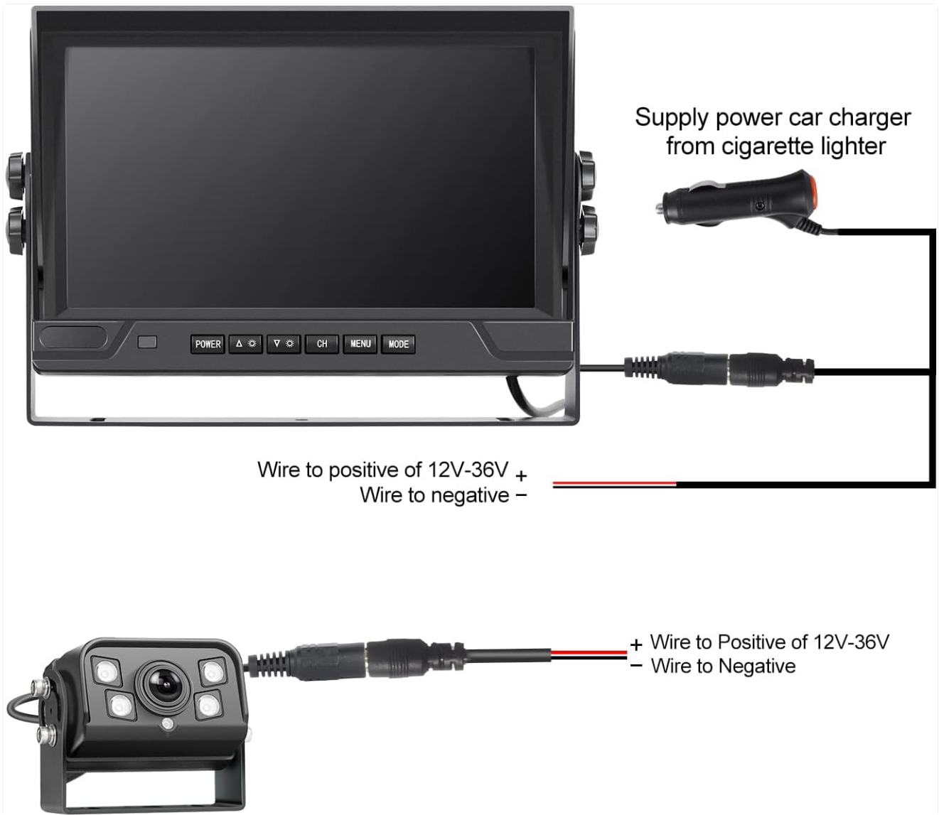
Image: A diagram illustrating the power connection methods for the monitor and cameras, including using a cigarette lighter adapter or direct wiring to 12V-36V power.
