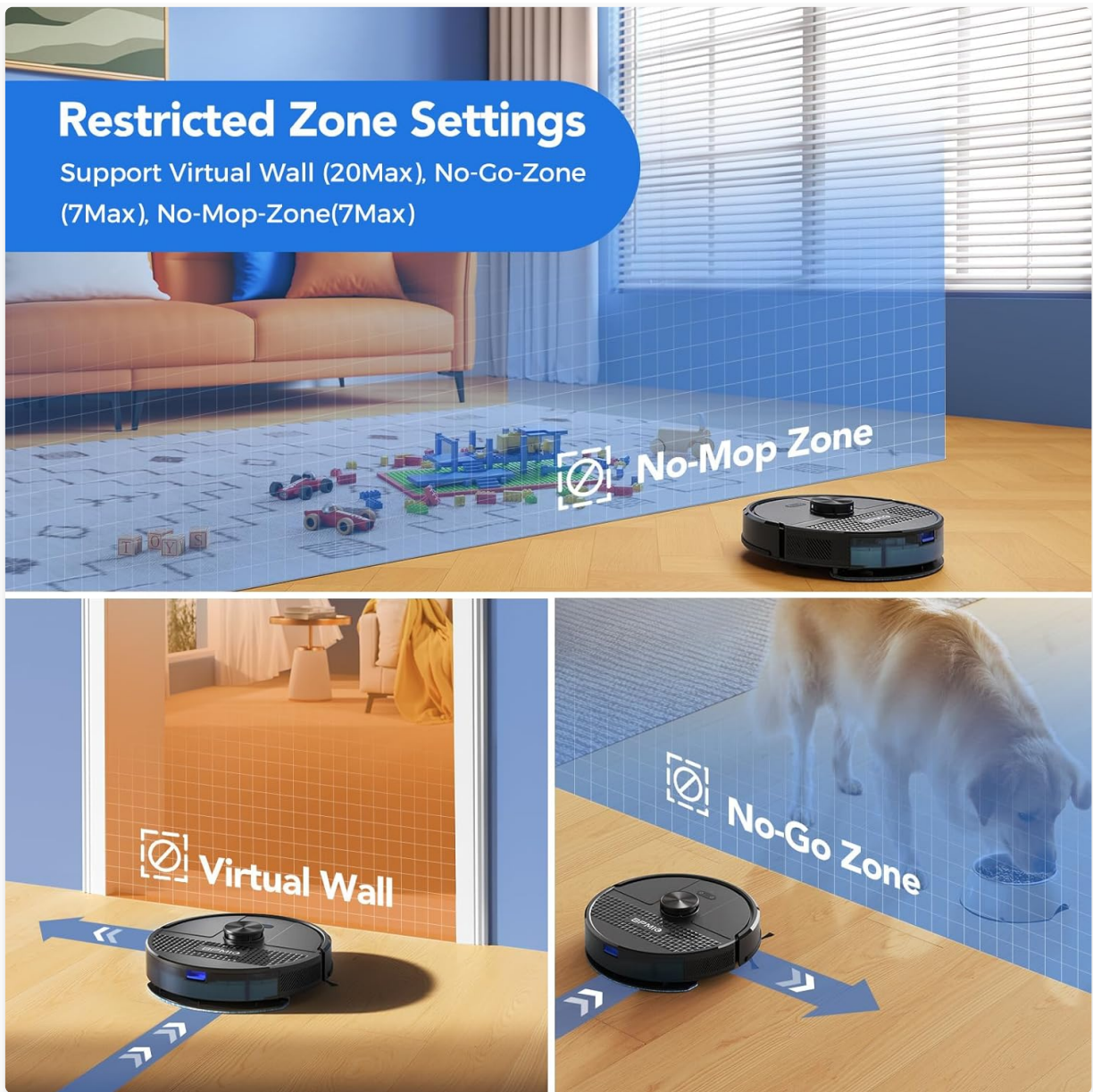
Image 4.3: Examples of setting restricted zones, including virtual walls and no-mop zones, within the app.
