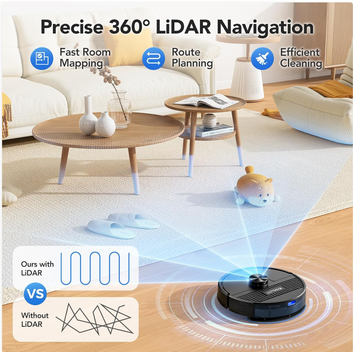
Image 2.2: Visual representation of the robot's 360° LiDAR navigation system, enabling precise mapping and route planning.
