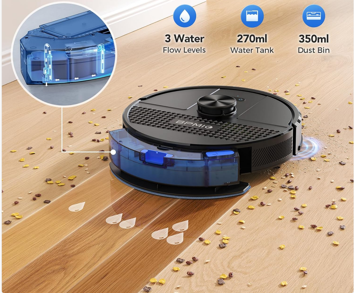
Image 2.3: The robot vacuum performing both vacuuming and mopping functions, highlighting its integrated water tank and dustbin.
